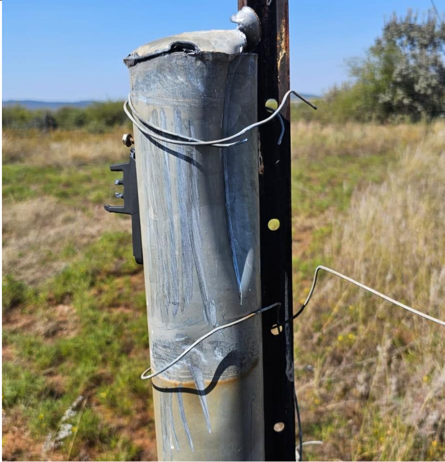
Figure 4: The propeller blade strike marks on the fence post.
