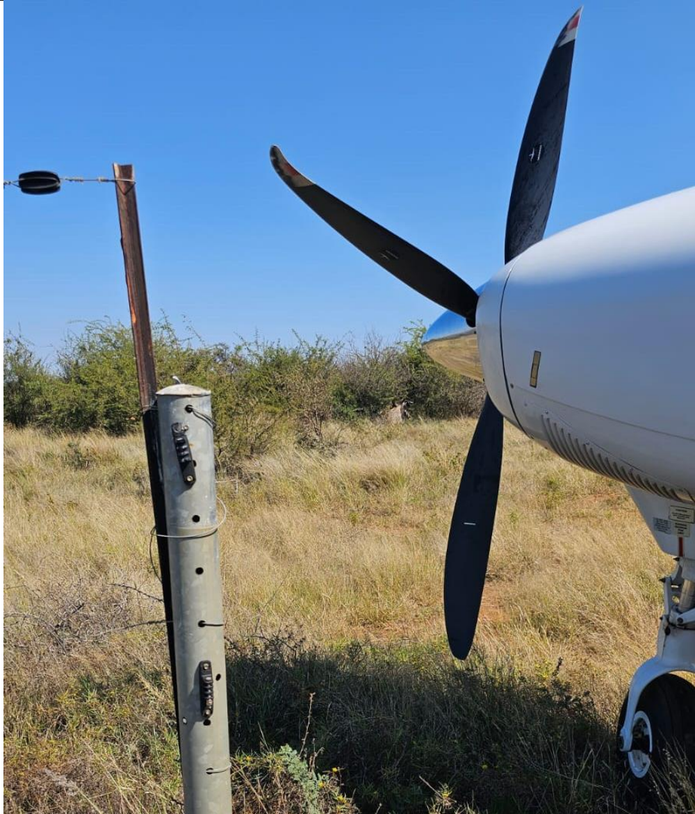
Figure 2: The steel fence post impacted by the propeller.
