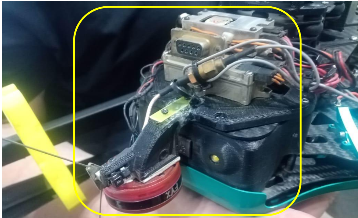
Figure 3: The transponder and antenna unit that was attached to the UAS are depicted in the yellow window. The picture was taken with the UAS in an inverted attitude. (Source: Operator)
