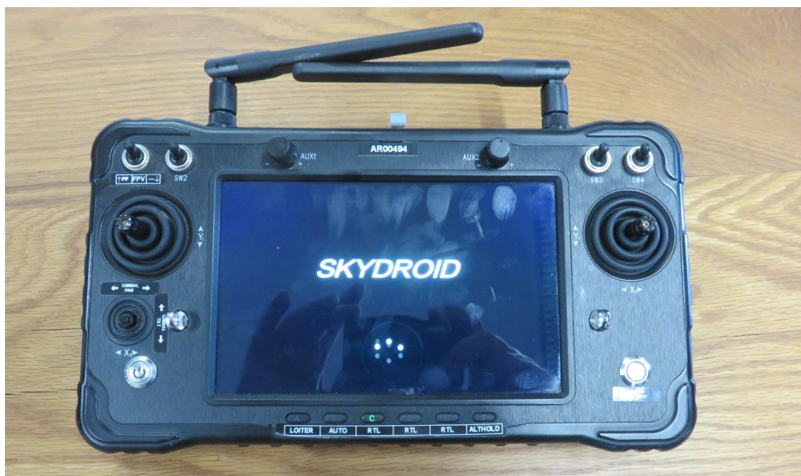
Figure 6: The Sirin remote pilot station with the RTL buttons below the display screen.
