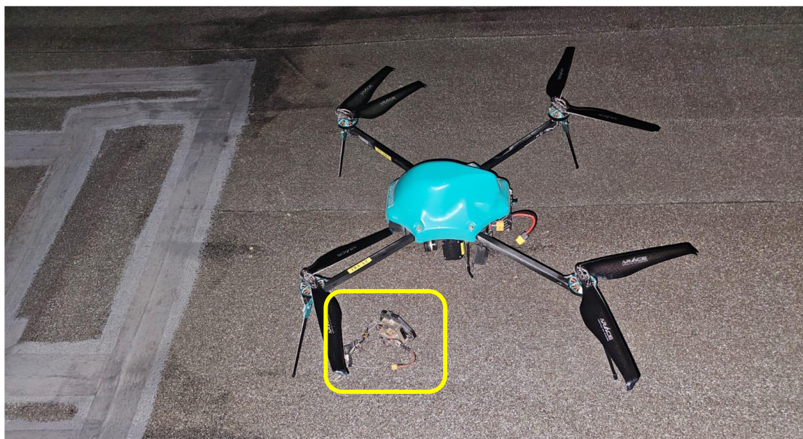
Figure 2: The transponder unit (in the yellow window) that dislodged from the UAS. (Source: Operator)
