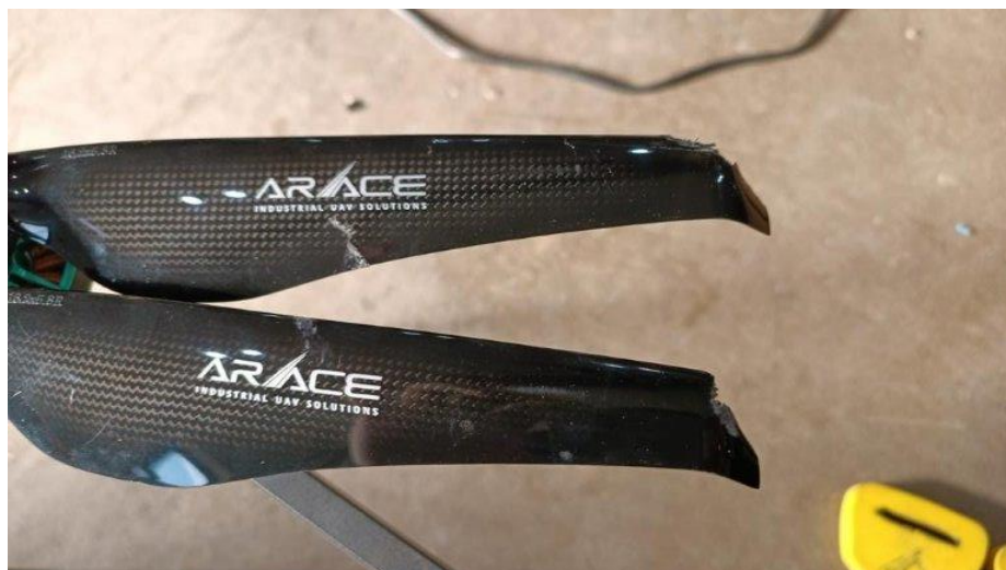
Figure 2: Damage to propellers was caused by contact with the loose tracking device. (Source: Araceuas.com)
