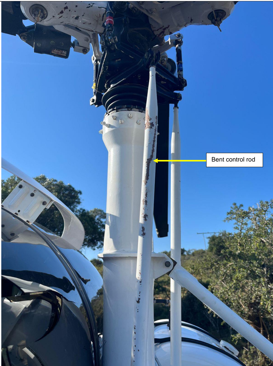
Figure 6: One of the control rods that was bent after impact with the power lines. (Source: Pilot)
