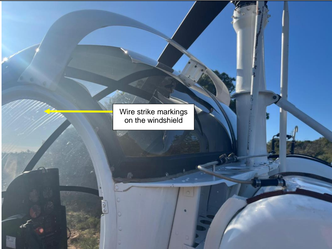
Figure 2: The wire strike markings on the windshield. (Source: Pilot)
