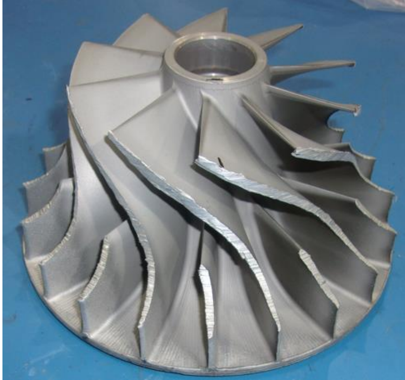
Figure 11: Second stage turbine rotor with damaged blades.
