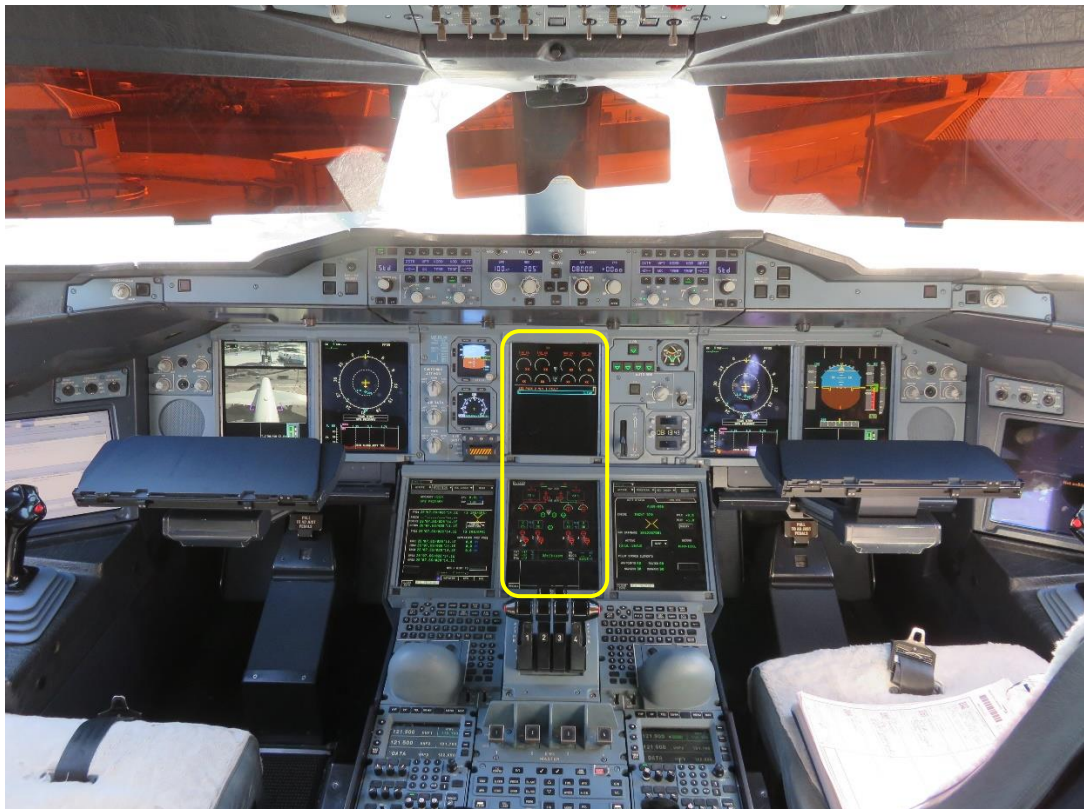
Figure 14: ECAM displayed in the yellow window in the cockpit of the Airbus A380, G-XLEH.
