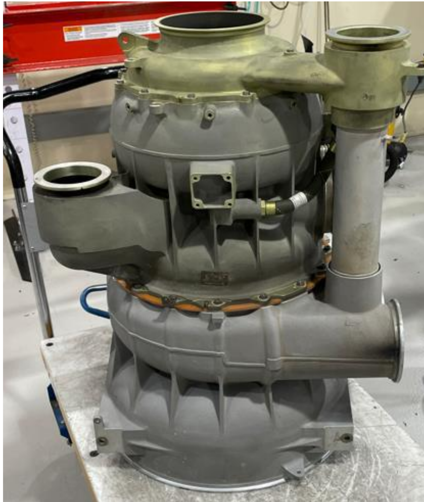
Figure 6: The ACM unit before disassembly.
