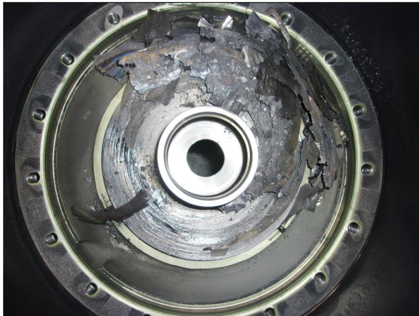
Figure 12: The turbine side thrust bearing was severely damaged during failure. The compressor side thrust bearing was similarly damaged, but as the turbine end shaft could not be removed, an image of that thrust bearing is not available.
