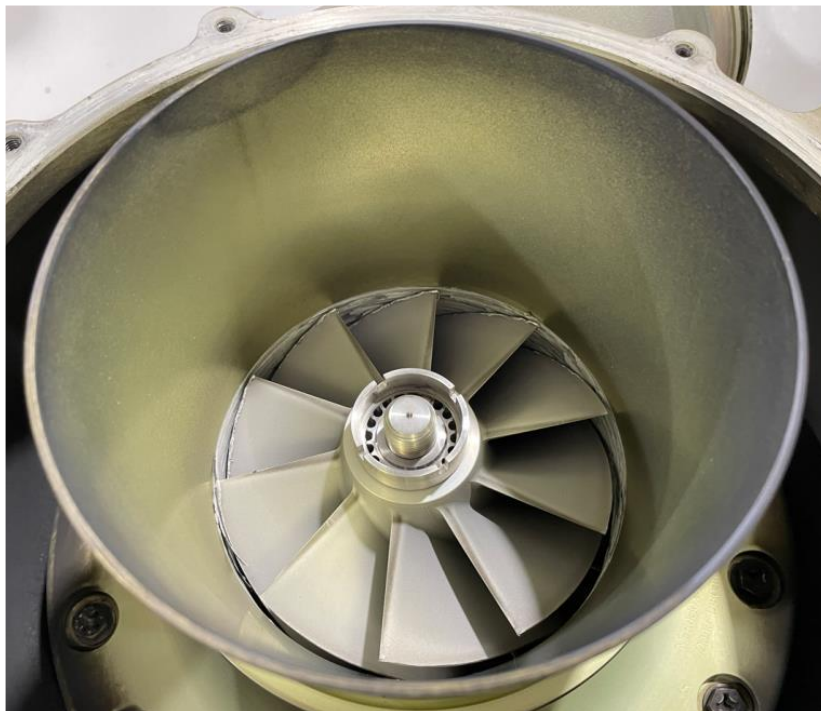
Figure 10: The second stage turbine rotor with radial damage.
