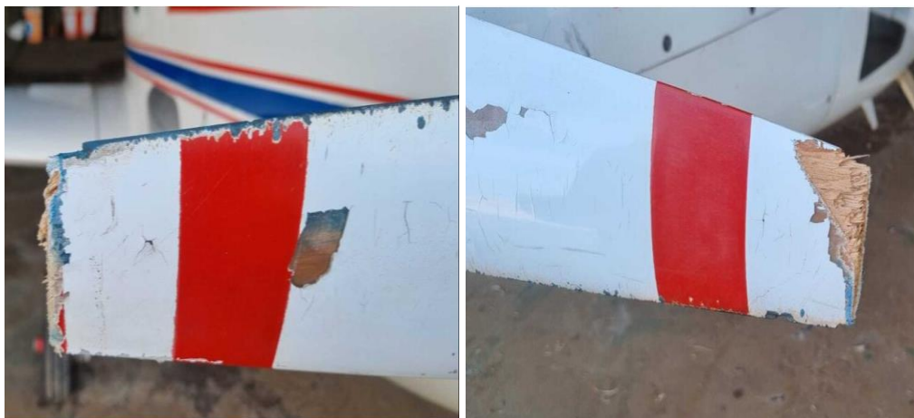
Figures 2 and 3: Damage sustained by the propeller blade tips. (Source: Pilot)
