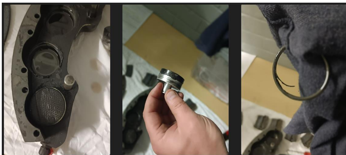
Figure 7: Brake calliper's third piston and the O-ring.
