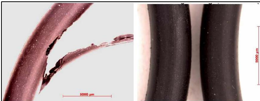
Figure 9: Damaged O-ring (left) and a comparison of new and used O-ring surfaces (right).
