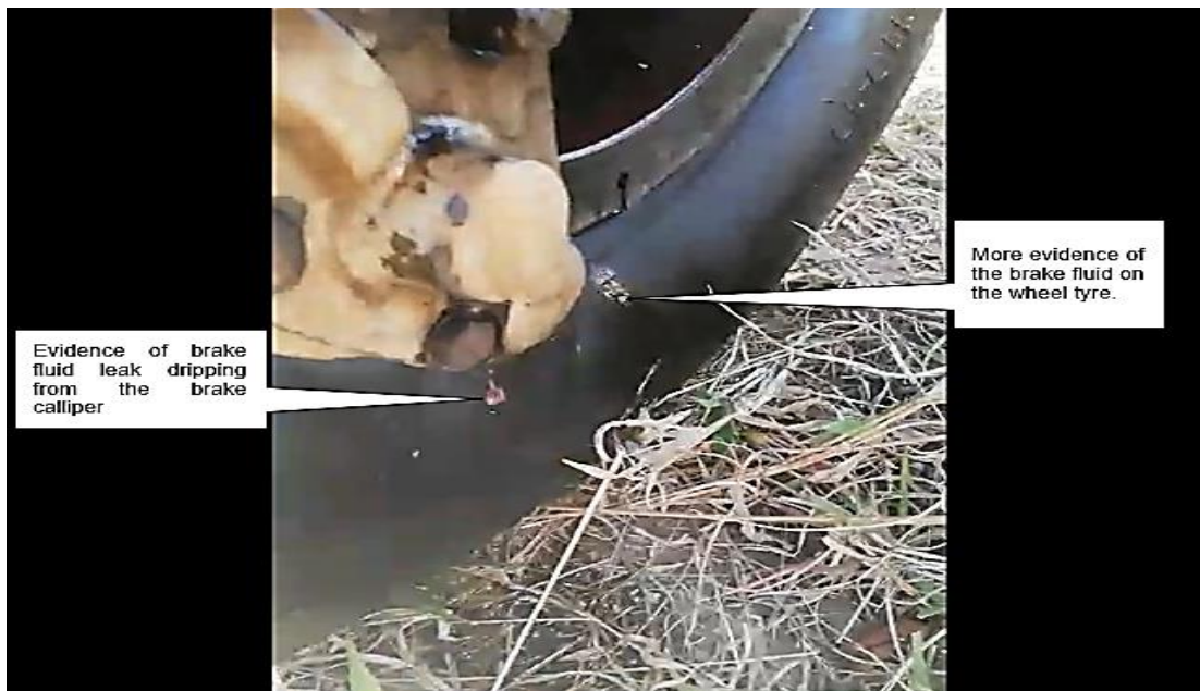
Figure 3: A snapshot taken from the video footage. It shows the brake fluid leaking from the brake calliper, and evidence of brake fluid on the tyre. (Source: PIC)
