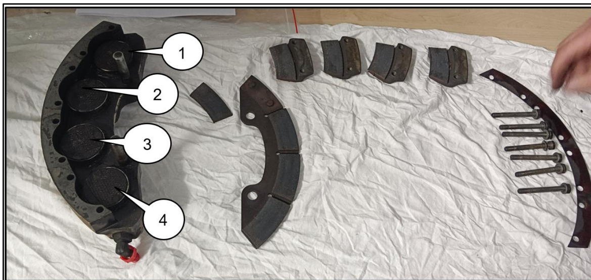
Figure 6: The brake calliper components with numbers pointing to the brake cylinder pistons.
