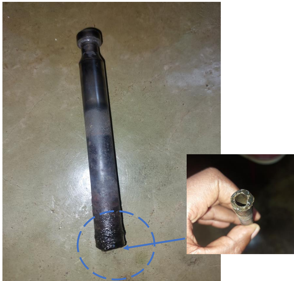
Figure 3: Cylinder number 2 exhaust valve stem with the head missing. It fractured during operation.
