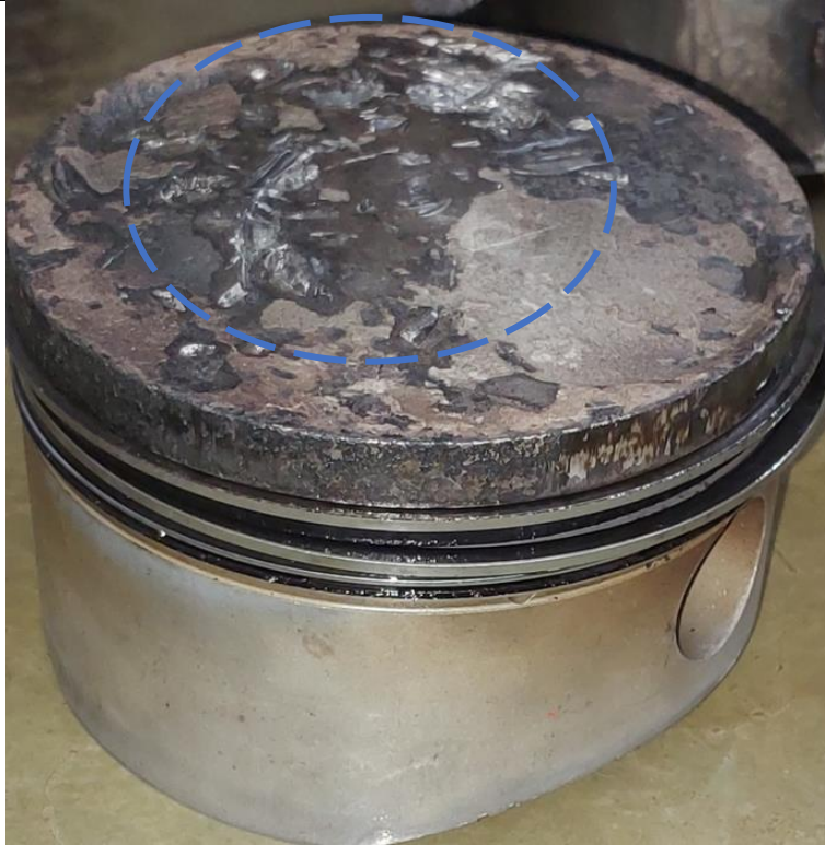
Figure 2: The blue circle indicates damage caused by the valve head on the number 2 piston crown.
