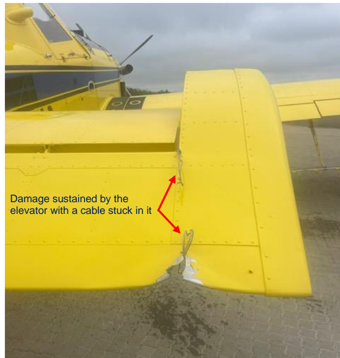
Figure 2: Damaged right-side elevator. (Source: Operator)
