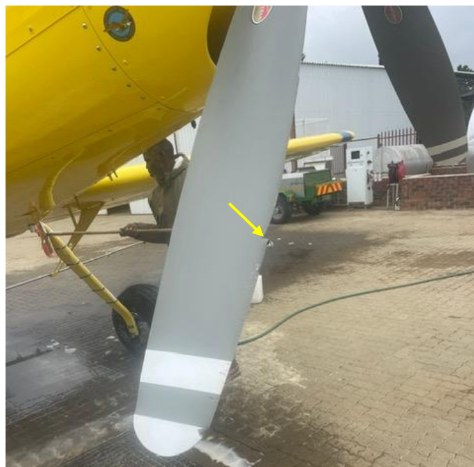
Figure 1: Damage on one of the blades leading-edge tip. (Source: Operator)
