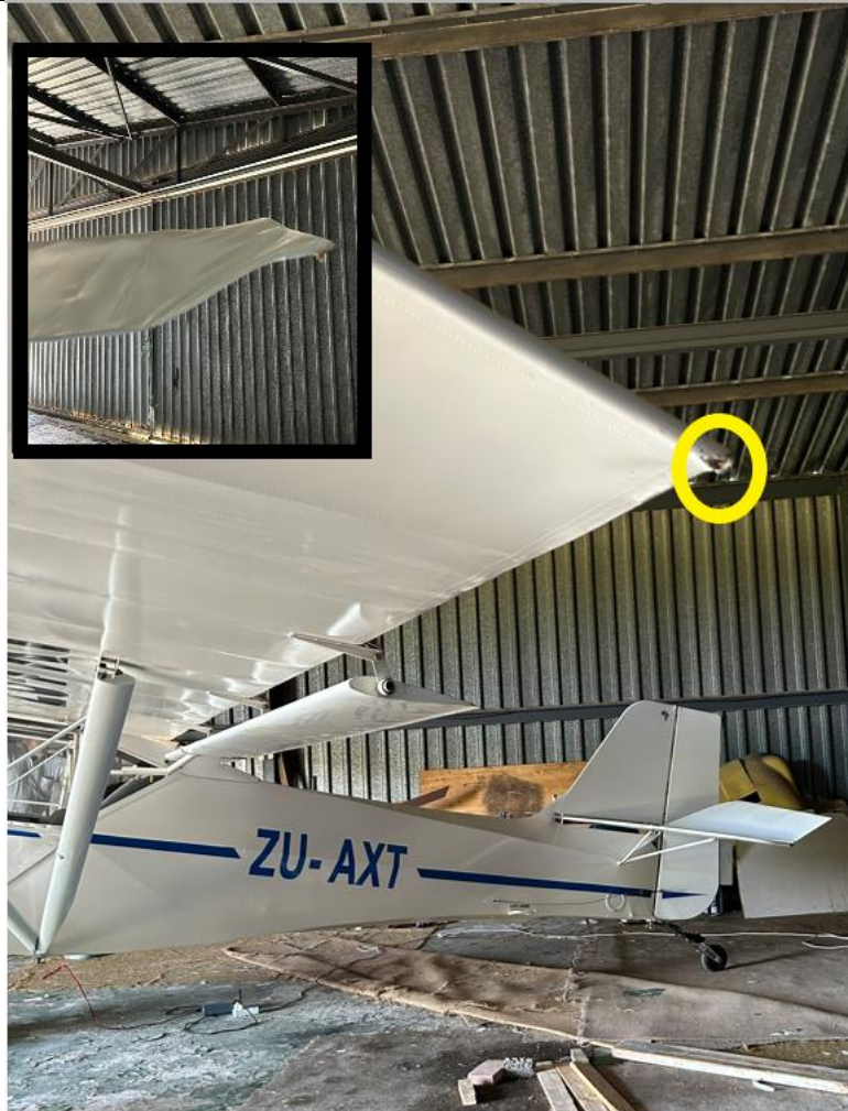
Figure 1: Damage on the left-wing tip. The inset shows the bent right wing tip in an upward direction. (Source: Operator)
