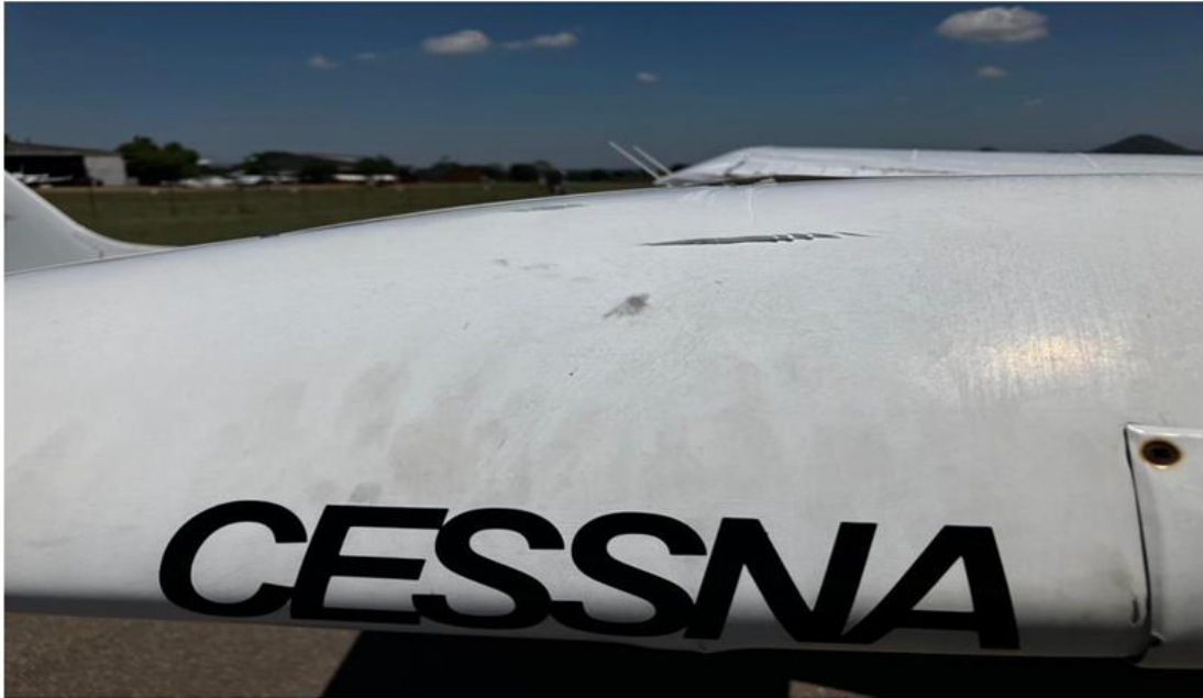
Figure 2: Minor damage to the right-wing tip fairing of ZS-SLY. (Source: ATO)
