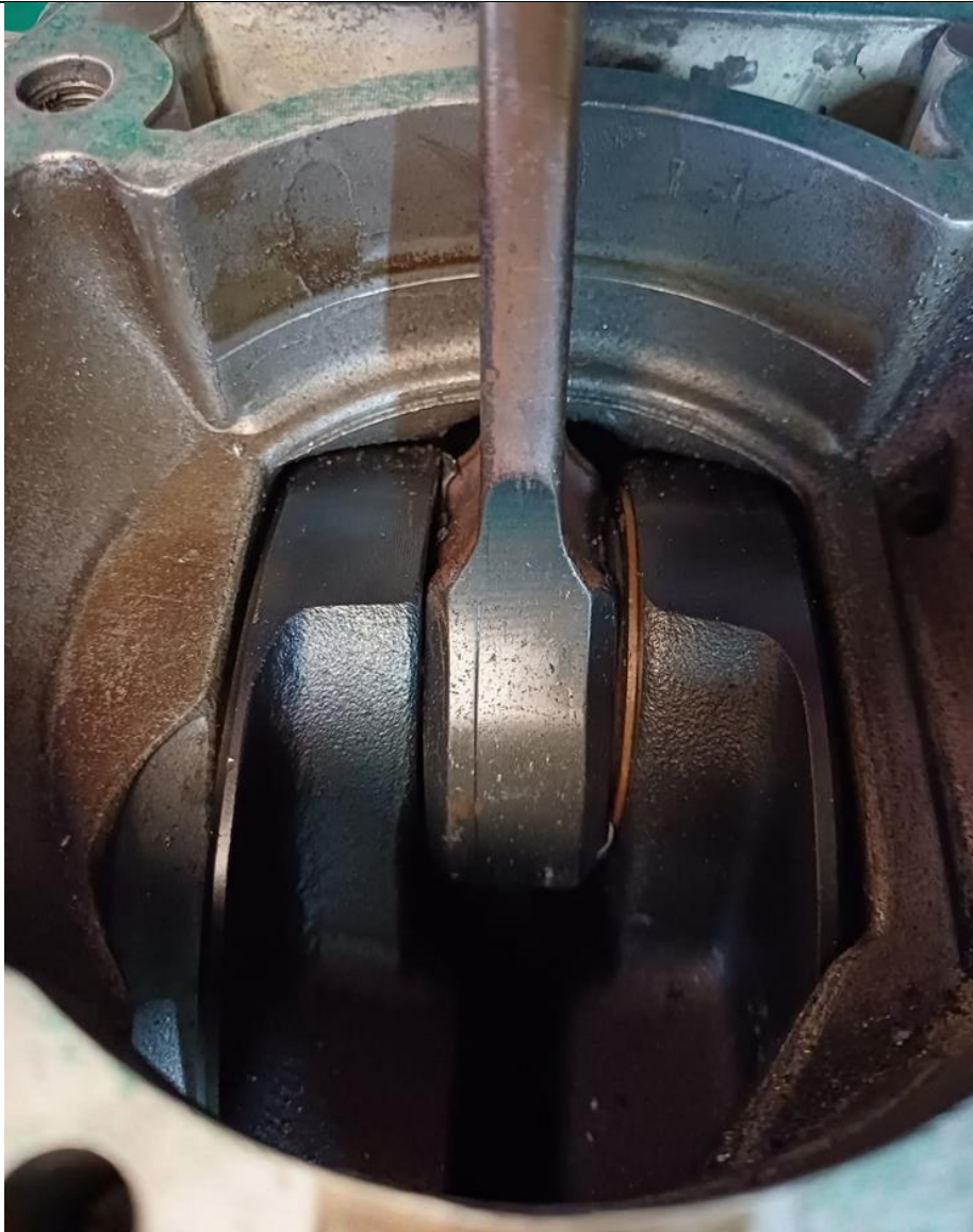
Figure 3: The worn number 2 cylinder conrod. (Source: Pilot)
