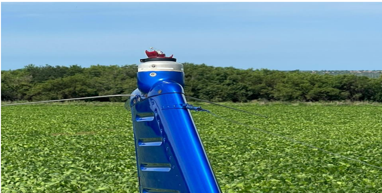
Figure 3: The damaged strobe light. (Source: Operator)
