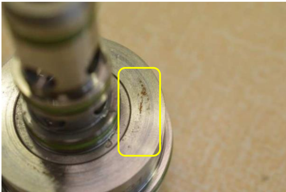
Figure 7: Corrosion on the main metering valve.
