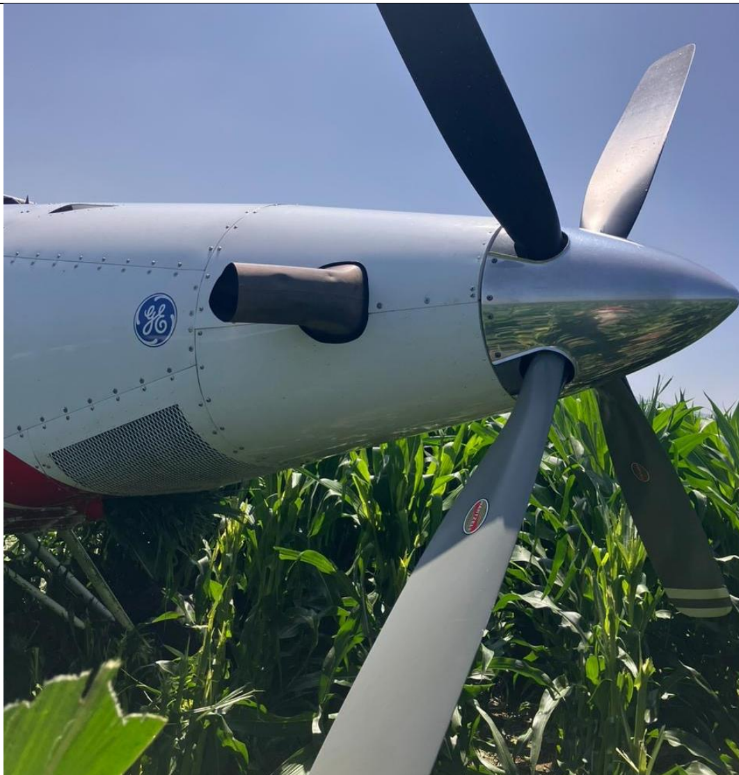
Figure 5: A view of the aircraft with the propeller in the feathered position. (Source: Pilot)
