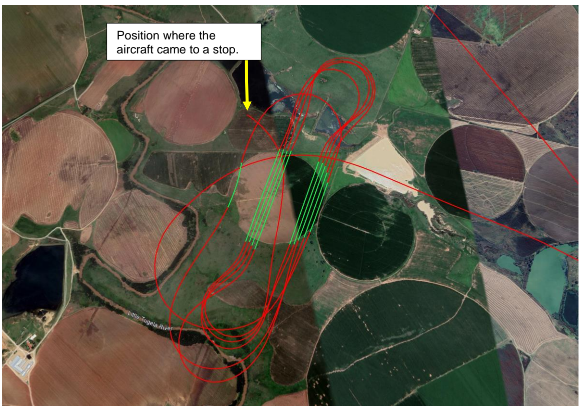
Figure 1: The spray pattern flown by the pilot, including the forced landing circuit. (Source: Pilot)
