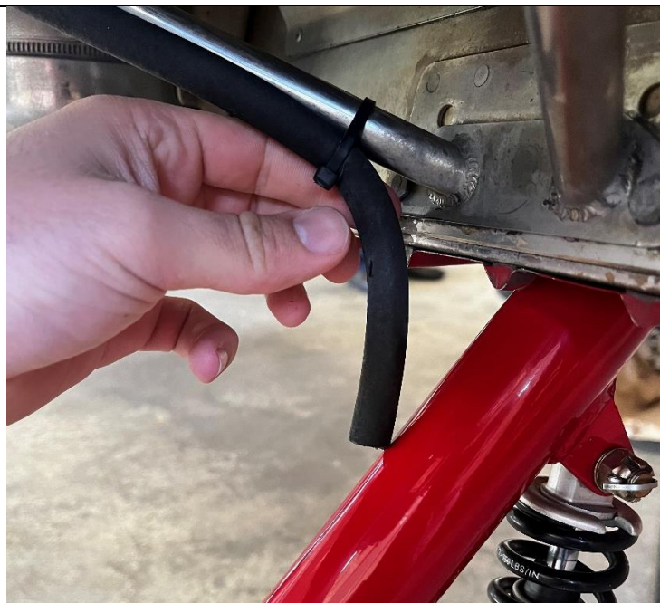
Figure 4: The fuel vent pipe. (Source: Operator)
