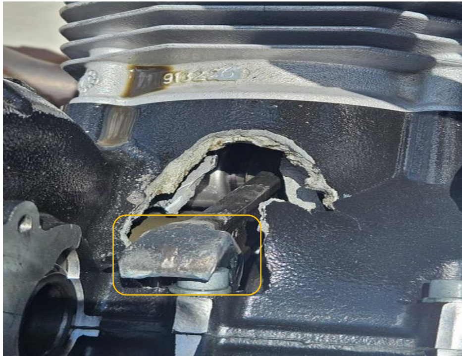
Figure 2: The Number 1 connecting rod protrudes from the crankcase. (Source: Flight instructor)
