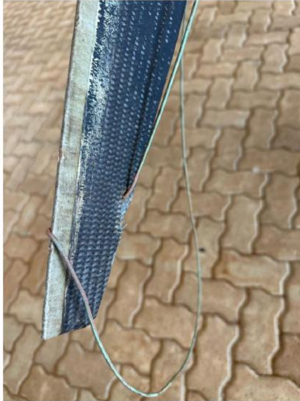
Figure 3: Damage to the propeller tip with the wire still entangled. (Source: Pilot)
