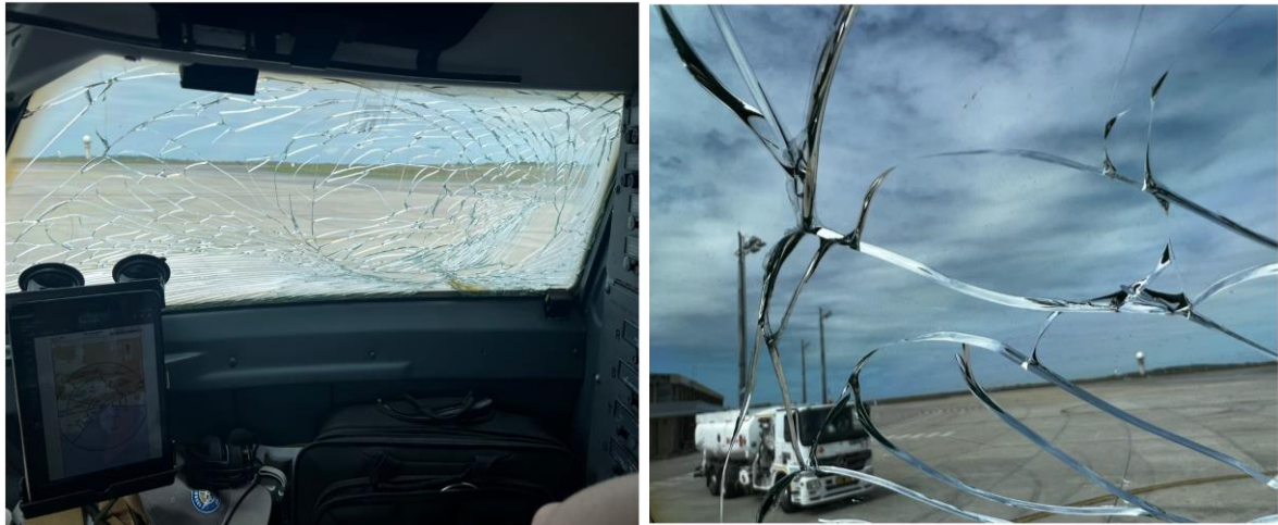
Figures 1 and 2: The cracked right-side windshield. (Source: Operator)
