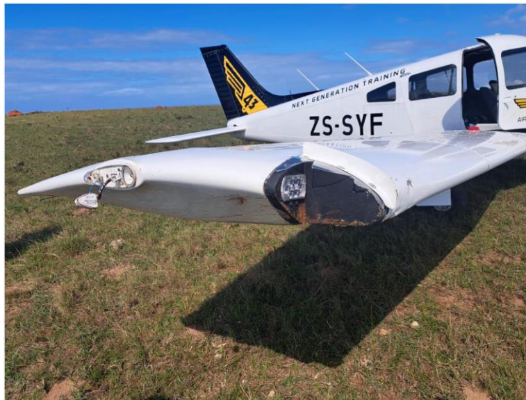
Figure 1: Damage after impact with an anthill during landing. (Source: Operator)
