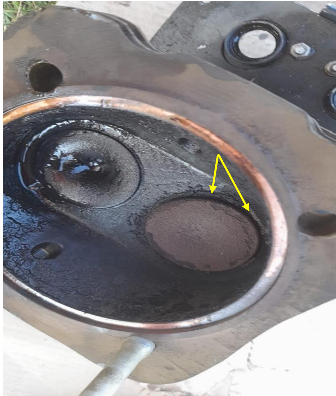
Figure 3: The partially opened No. 3-cylinder exhaust valve. (Source: Operator)
