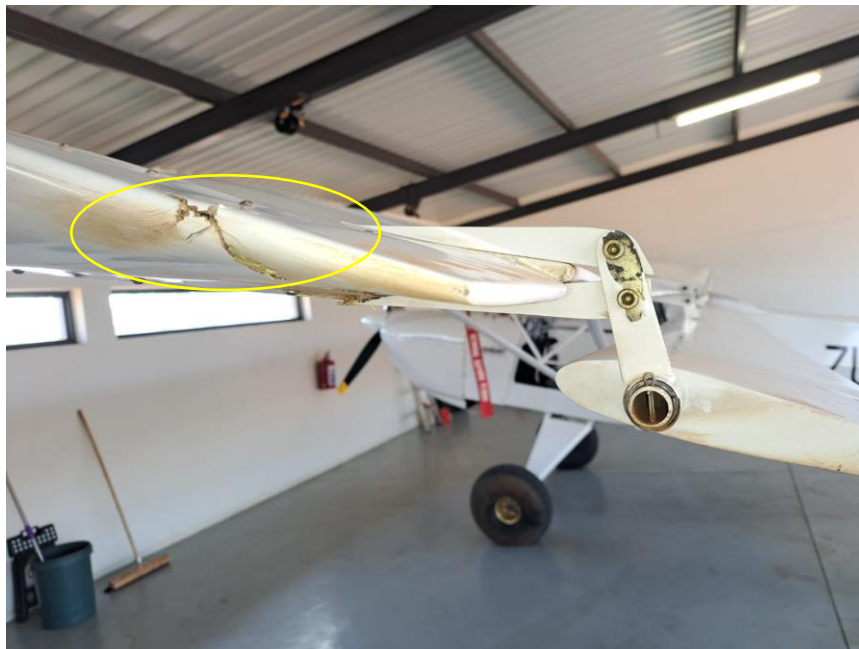
Figure 2: The aircraft after it was recovered to the hangar at the airstrip. The yellow circle shows the damaged left-wing tip fairing. (Source: Pilot)
