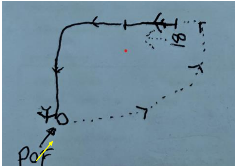
Figure 1: The pilot's sketch depicts the take-off direction and the point at which the exhaust outlet pipe-end part broke off after executing a left turn. (Source: Pilot)
