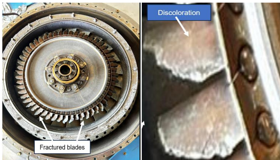
Figures 6 and 7: Fractured axial turbine rotor blades (left picture). Discolouration on the turbine axial rotor blades (right picture).
