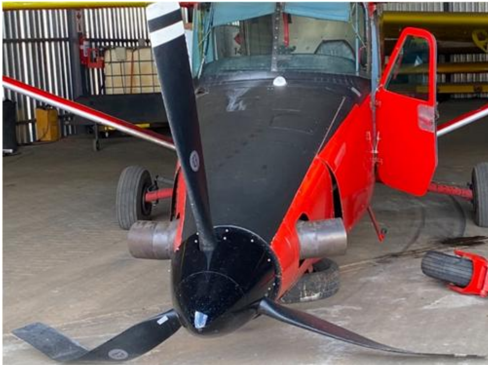
Figure 5: The damaged propeller blades.
