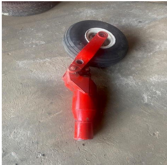
Figure 4: The severed nose gear.
