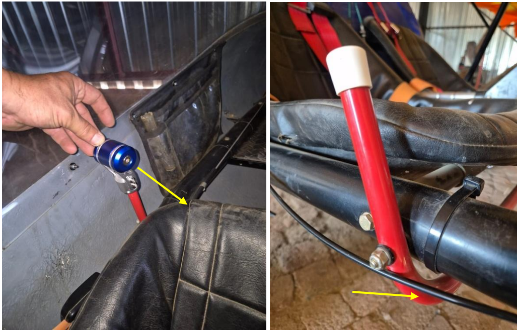
Figures 4 and 5: The throttle (left picture) on the left side of the pilot's seat. The throttle cables in the plastic sheath run from the left side of the pilot's seat to the engine (right picture). (Source: Pilot)
