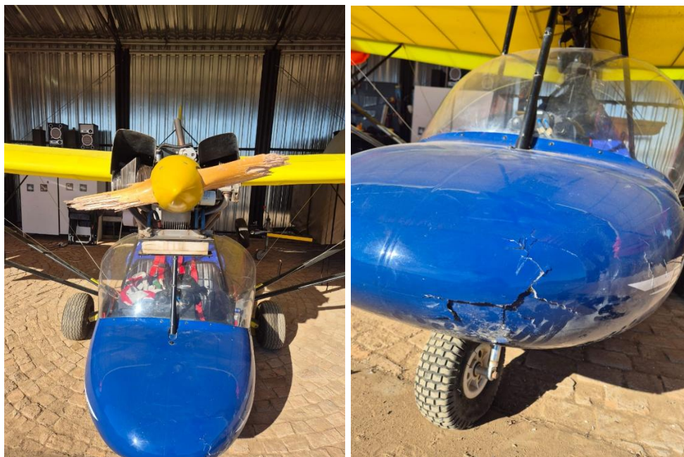
Figures 1 and 2: The damaged propeller (left) and the nose section's left lower composite structure (right). (Source: Pilot)
