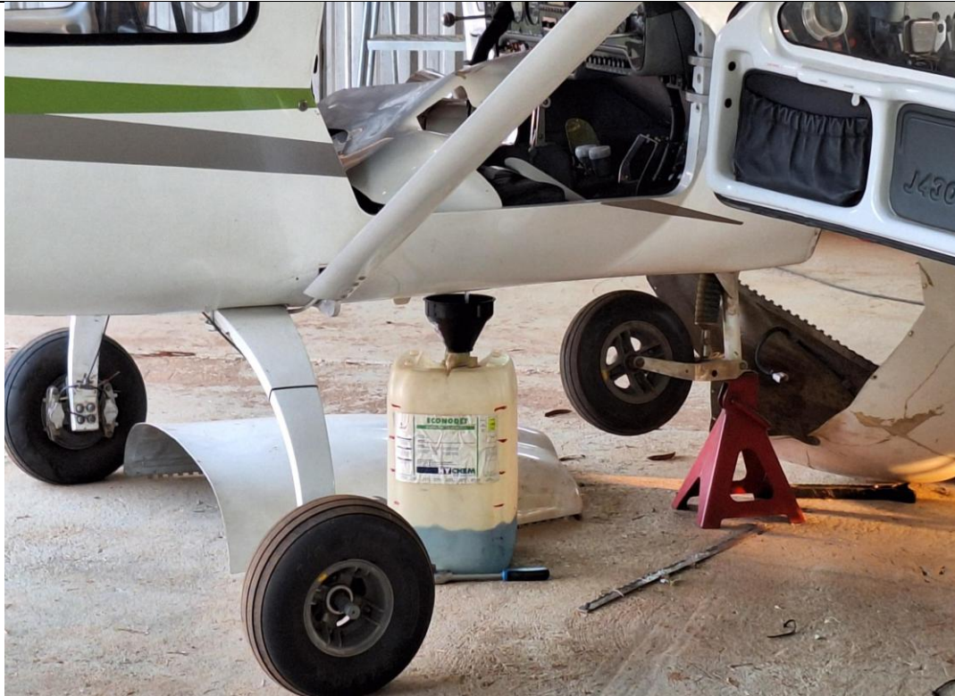
Figure 4: Fuel is drained through the quick-drain valve at the bottom of the header tank.
