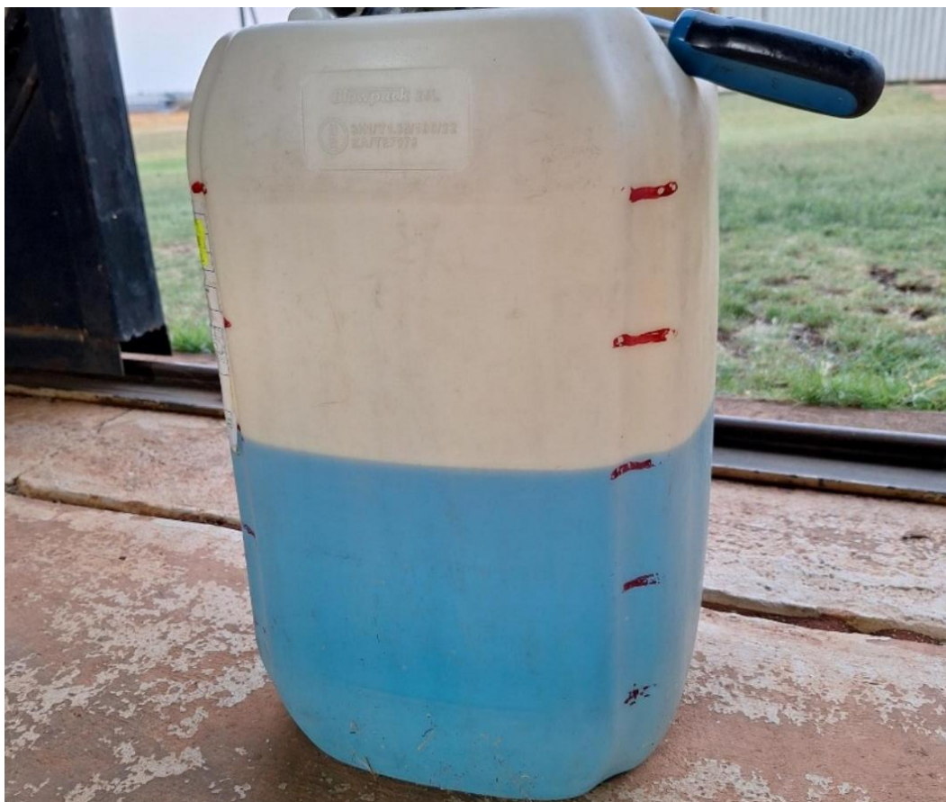
Figure 5: The drained 15 litres of fuel.
