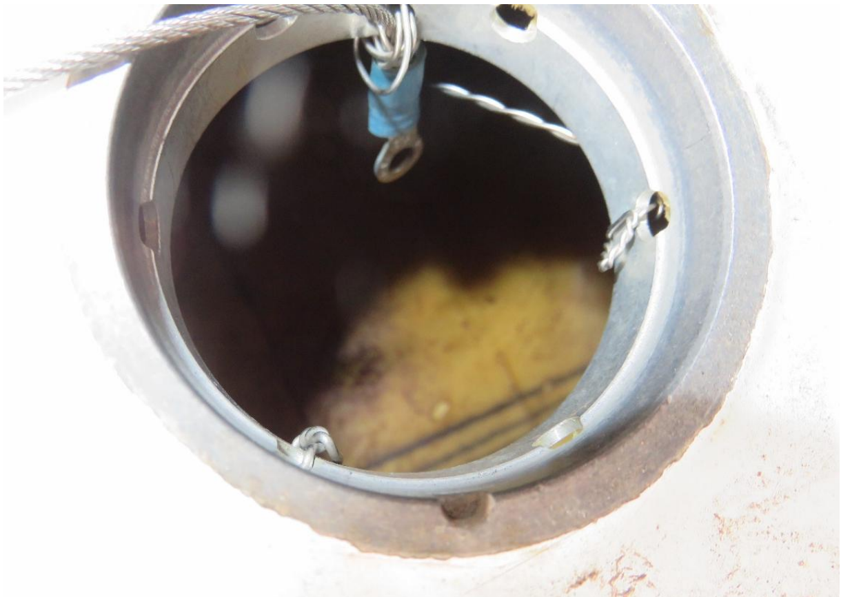
Figure 14: A photograph of the right-wing tank taken on 2 September 2025. The tank was empty after the fuel tank cap was removed.
