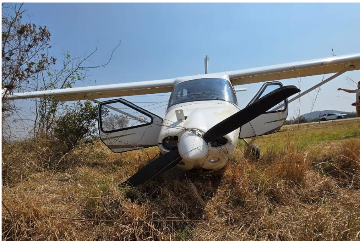
Figure 3: The barbed wire entangled around the propeller spinner and windshield. (Source: Pilot)
