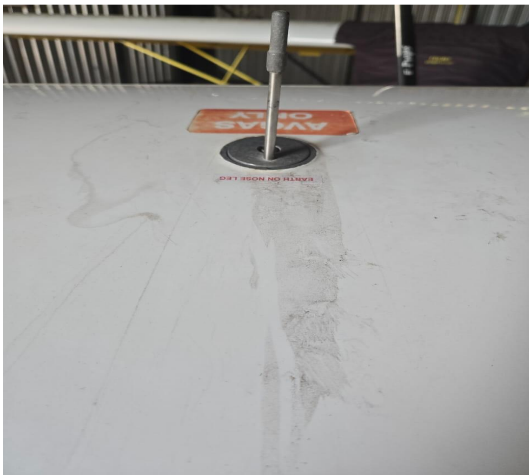
Figure 9: Fuel streak on top of the right wing indicates fuel leak from the wing tank. (This photo was taken on 2 September 2025, four days after the serious incident flight).
