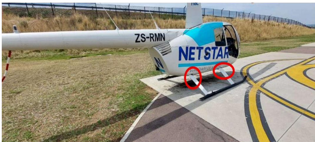
Figure 1: Red circles indicate minor damage on the helicopter's upper portions of the landing gear skids caused by overload. (Source: Operator)
