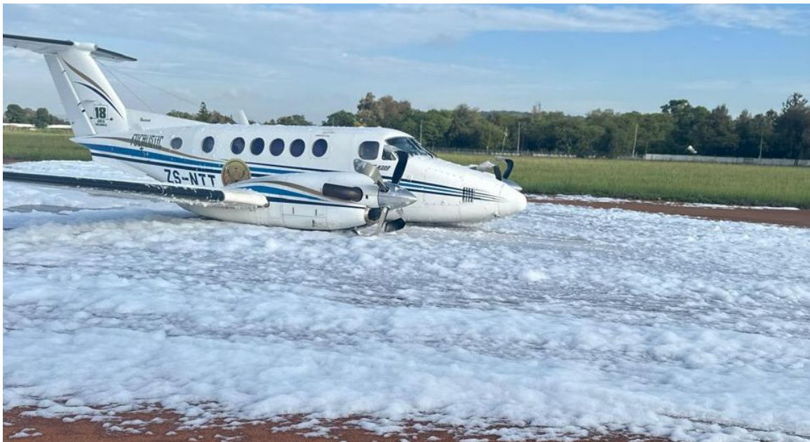
Figure 2: The fire-retardant foam sprayed on the runway during the serious incident. (Source: Operator)
