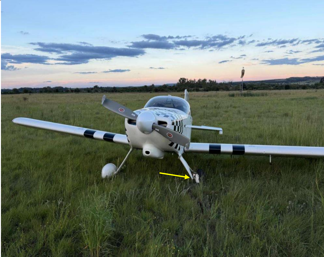
Figure 2: The aircraft with the bent left main landing gear at the serious incident site. (Source: Pilot)
