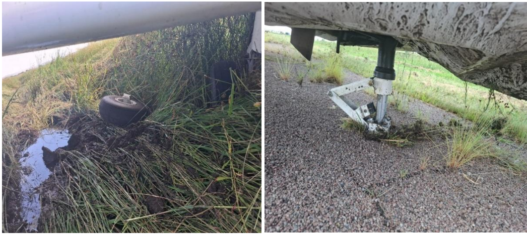
Figures 3 and 4: The broken bottom part of the nose gear with the nose wheel still secured to the axle (left picture). The top part of the nose gear strut with the torque link still attached to the oleo (right picture). (Source: Operator)
