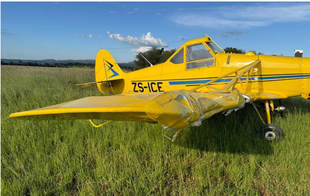
Figure 4: Damage to the right-wing leading edge. (Source: Pilot)
