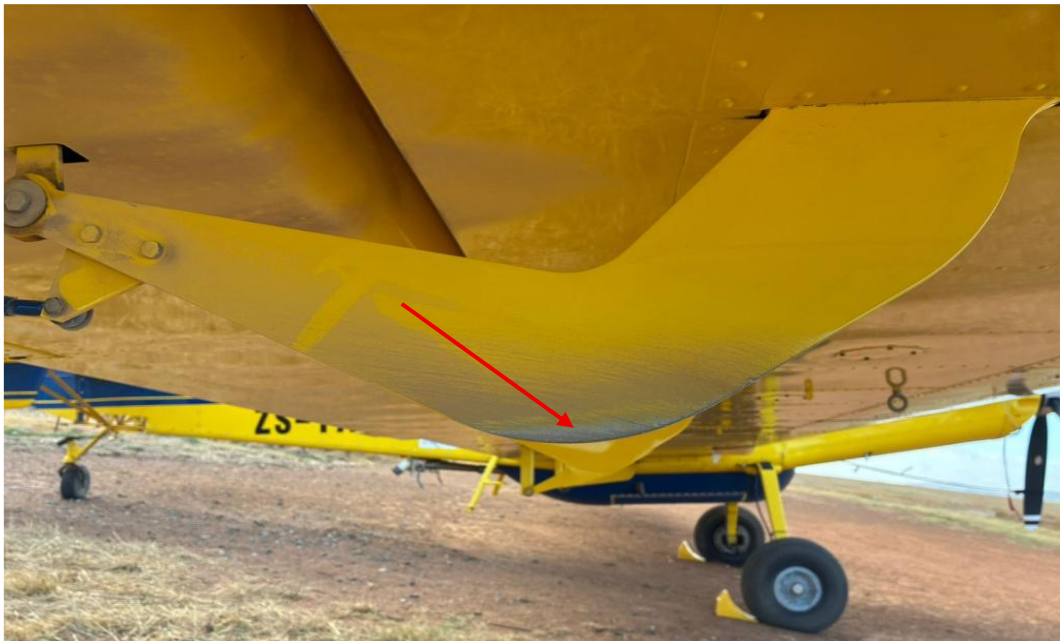
Figure 1: Chafing on the right-wing outer flap bracket (red arrow). (Source: Operator)
