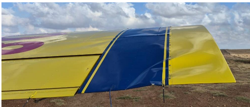
Figure 2: Dents on the right-wing tip trailing edge. (Source: Operator)
