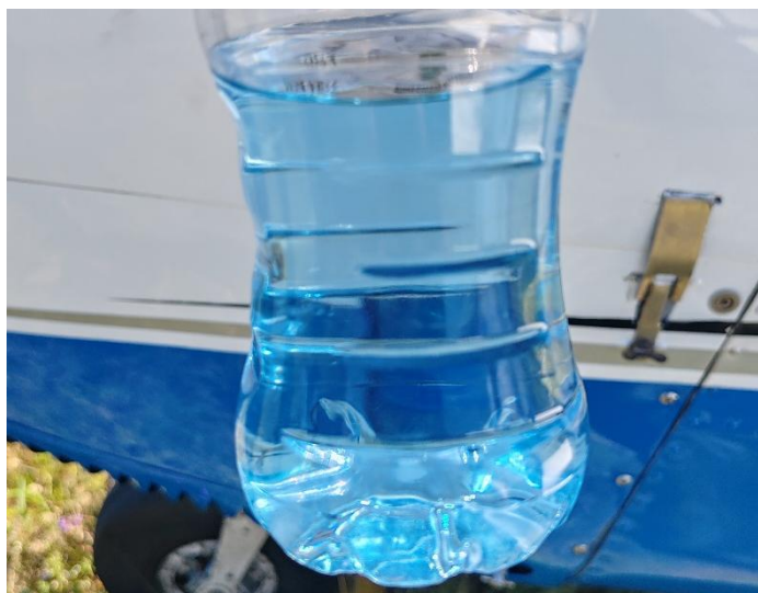
Figure 2: Fuel sample from the gascolator of ZS-SDR.
