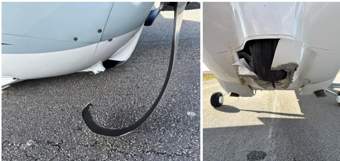
Figures 3 and 4: The propeller blade (left) and landing gear doors (right) that were damaged from abrasion with the runway. (Source: Pilot)
