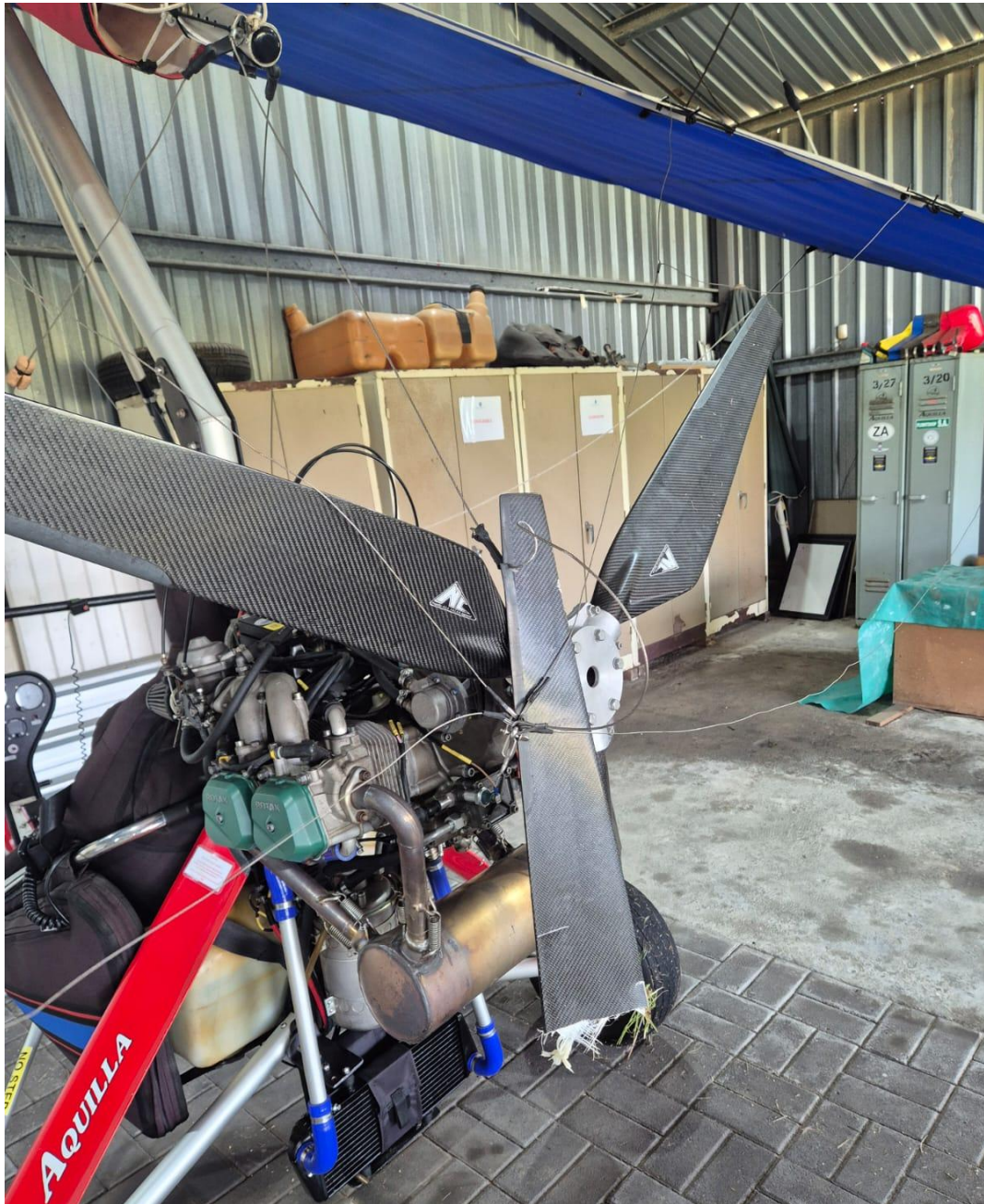
Figure 2: A singular broken propeller blade. (Source: Pilot)
