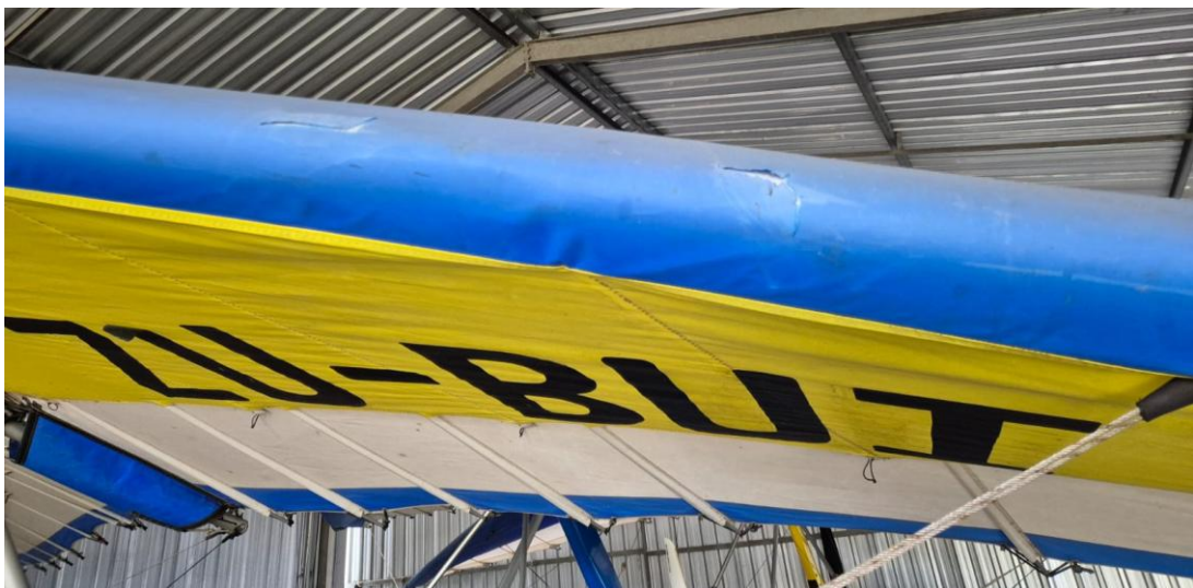
Figure 4: The leading-edge canvas covering of the ZU-BUI showing sustained damage. (Source: Pilot)
