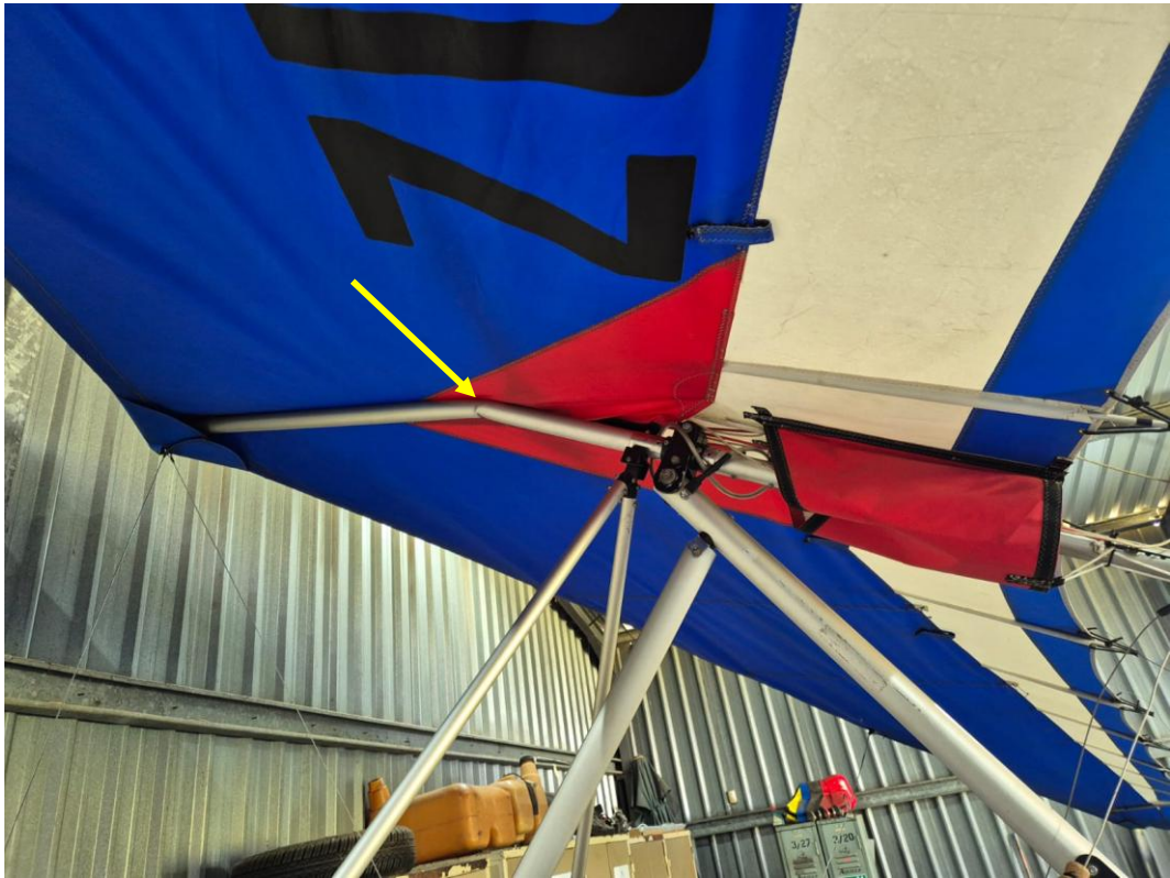
Figure 3: The bent keel tube. (Source: Pilot)
