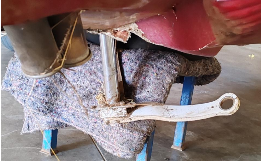
Figure 3: The damaged nose gear strut.
