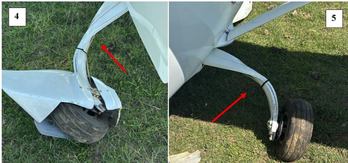
Figures 4 and 5: The damaged left and right landing gear (the red arrows point to the damage). (Source: Pilot)
