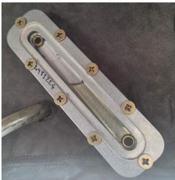
Figure 7: The wing fuel sight glass. (Source: Technical Report)
