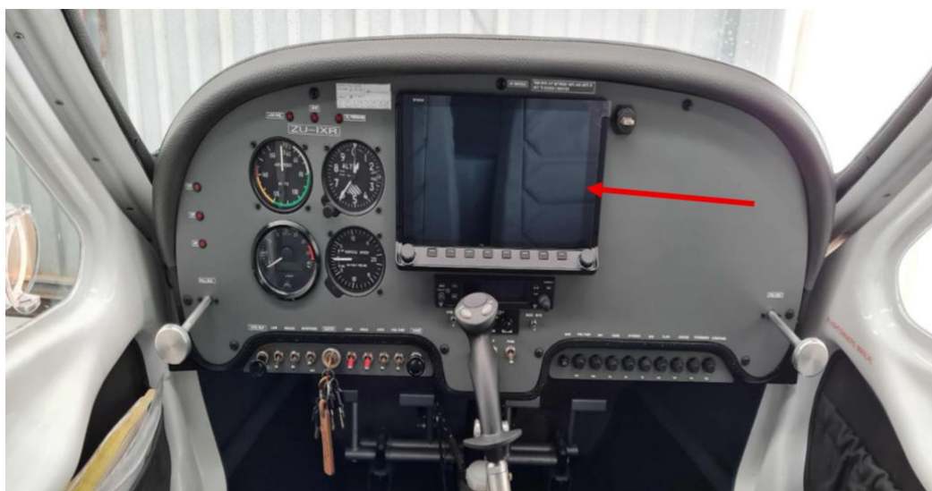
Figure 6: ZU- IXR instrument panel showing Dynon HDX Skyview EFIS (red arrow). (Source: Technical report)
