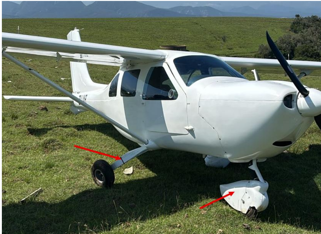
Figure 1: The damaged landing gear (red arrows). (Source: Pilot)
