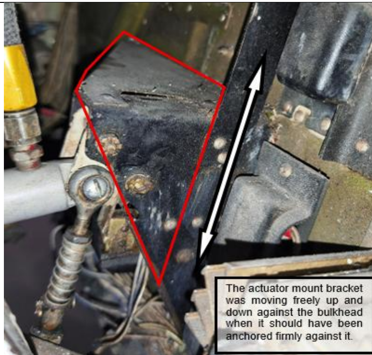
Figure 2: The loose actuator mount bracket on ZS-SNR.
