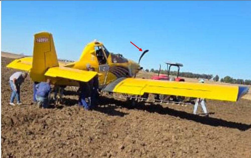
Figure 2: The aircraft in its final position at the serious incident site. The red arrow points to the damaged blades. (Source: Pilot)
