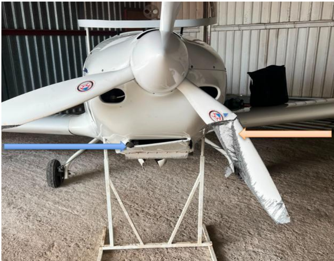
Figure 3: The amber arrow indicates the damaged propeller blade, and the blue arrow indicates the damaged cowling area. (Source: Pilot)
