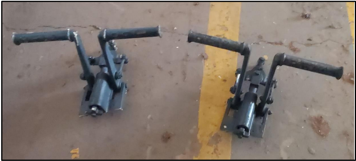
Figure 8: Both tail rotor pedals were found severed.
