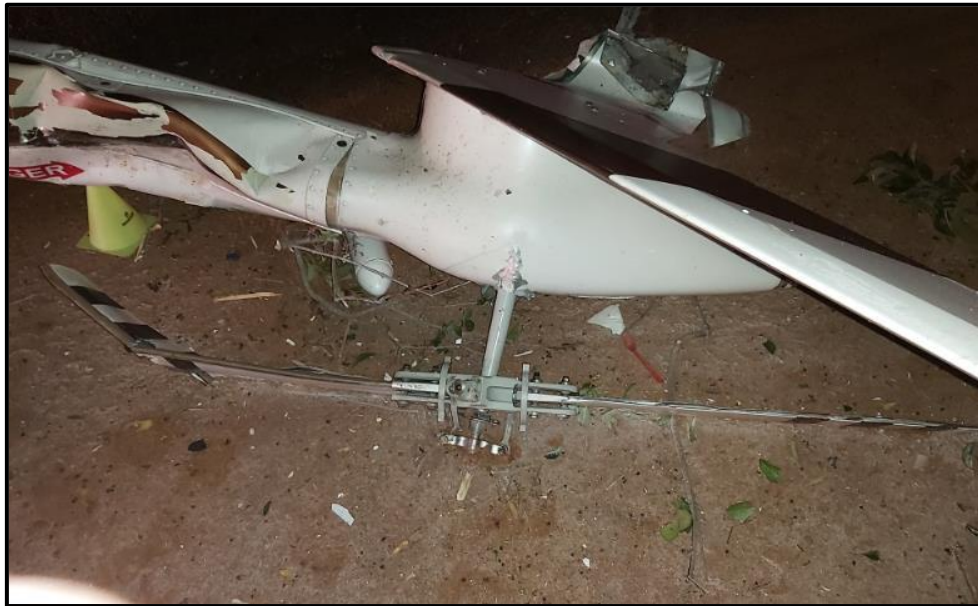
Figure 9: The tail rotor section after the accident.
