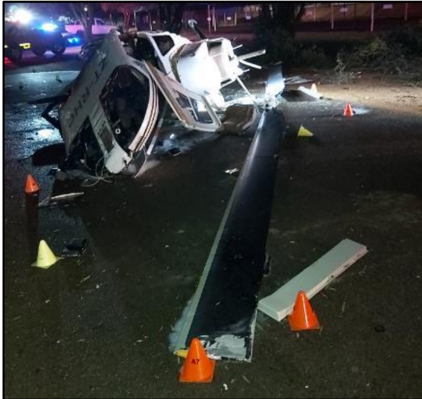
Figure 7: The main rotor blade assembly after the accident.
