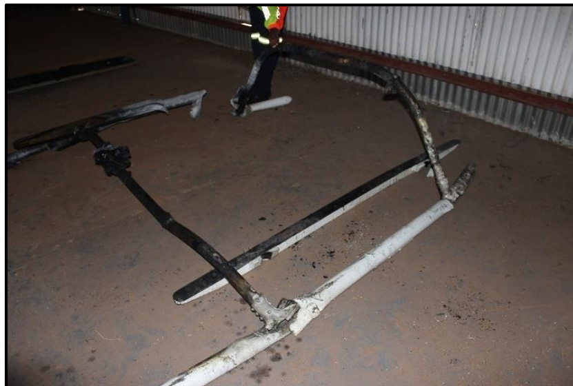
Figure 6: The skid gear assembly after the accident.
