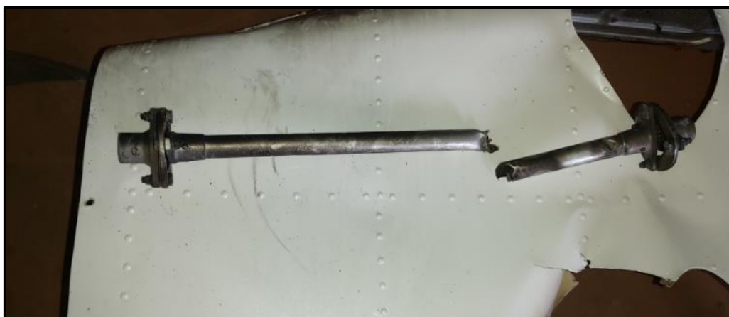
Figure 13: The damaged input shaft.
