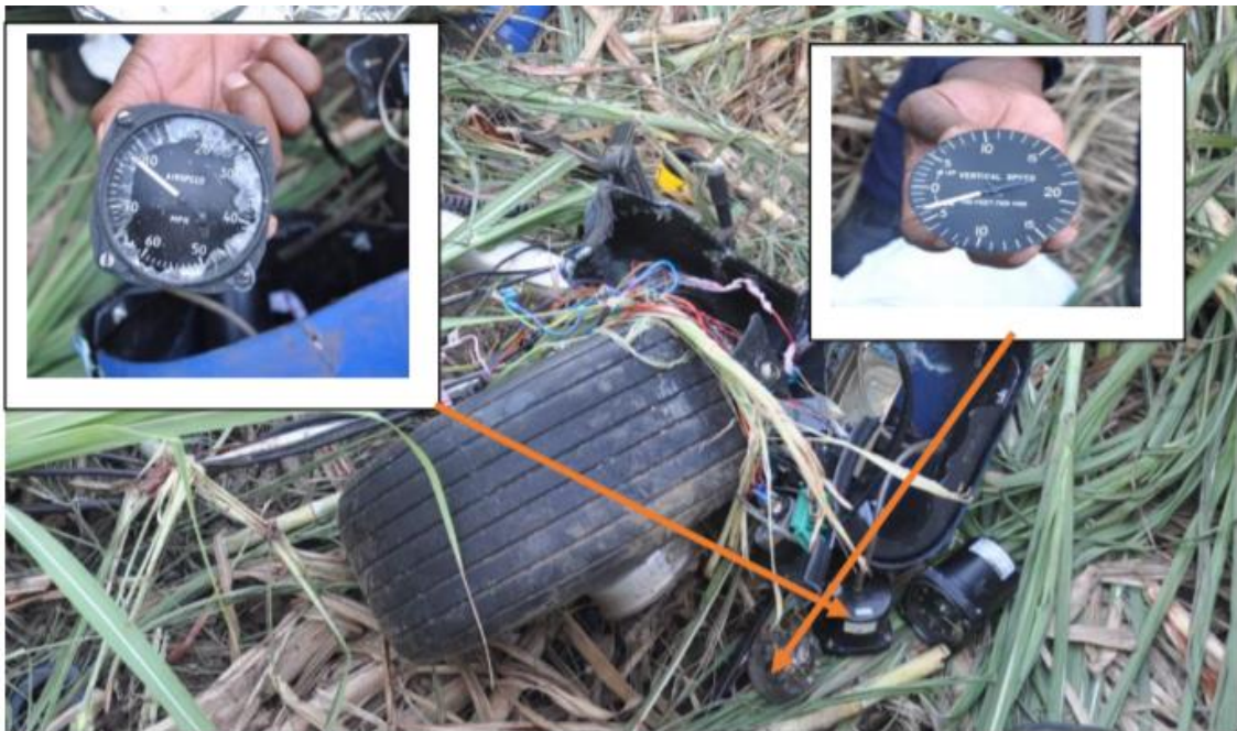
Figure 7: The damaged nose section. The left inset image shows airspeed indicator and the right inset image shows vertical speed indicator of the instrument panel.
