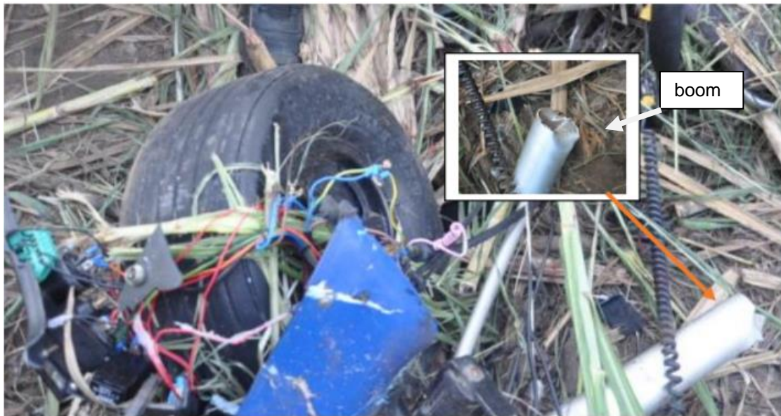
Figure 5: The boom that fractured and separated from the nose gear.
