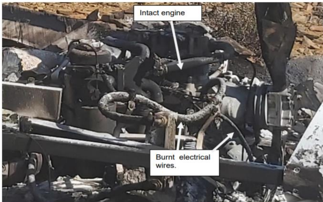
Figure 8: The engine was found still intact.
