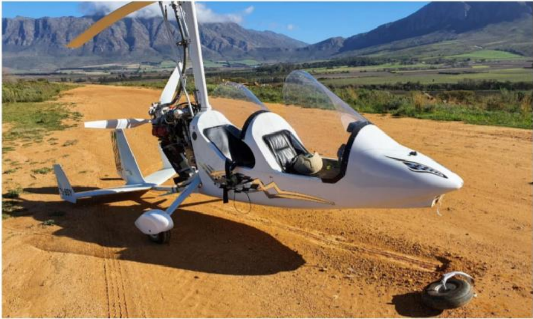
Figure 3: The picture of the ZS-BDY damaged nose landing gear sustained in the past accident that was not reported.
