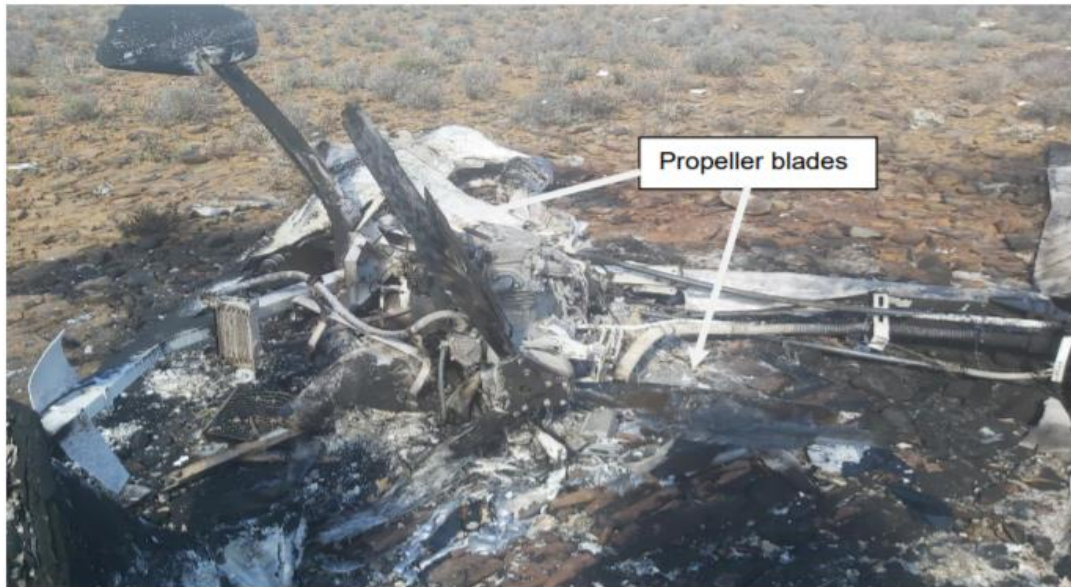
Figure 9: The burnt propeller blades.
