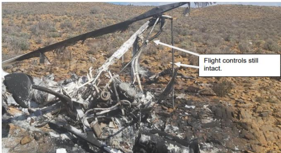
Figure 10: Continuity of flight controls still intact.
