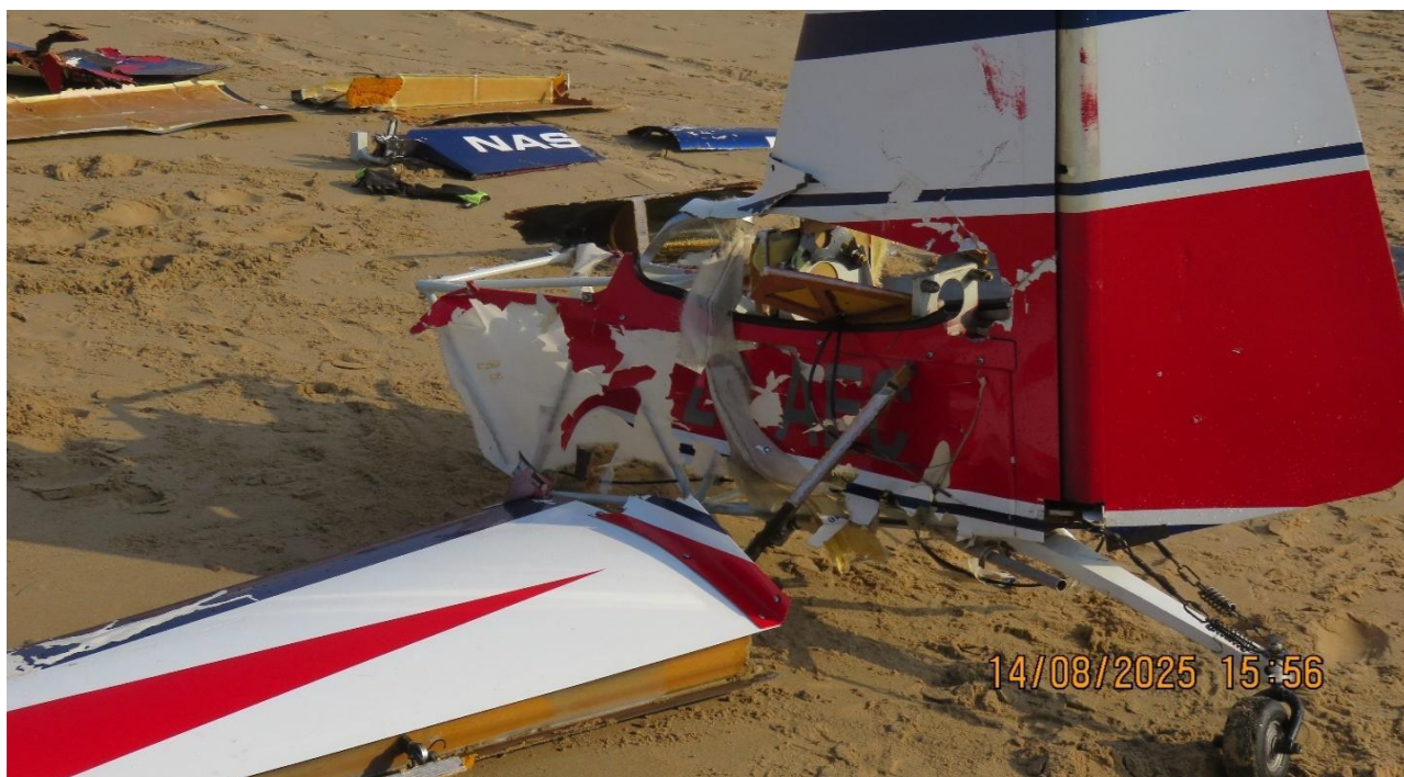
Figure 5: Reconstruction of the aircraft with elements that were recovered on the day of the accident.
