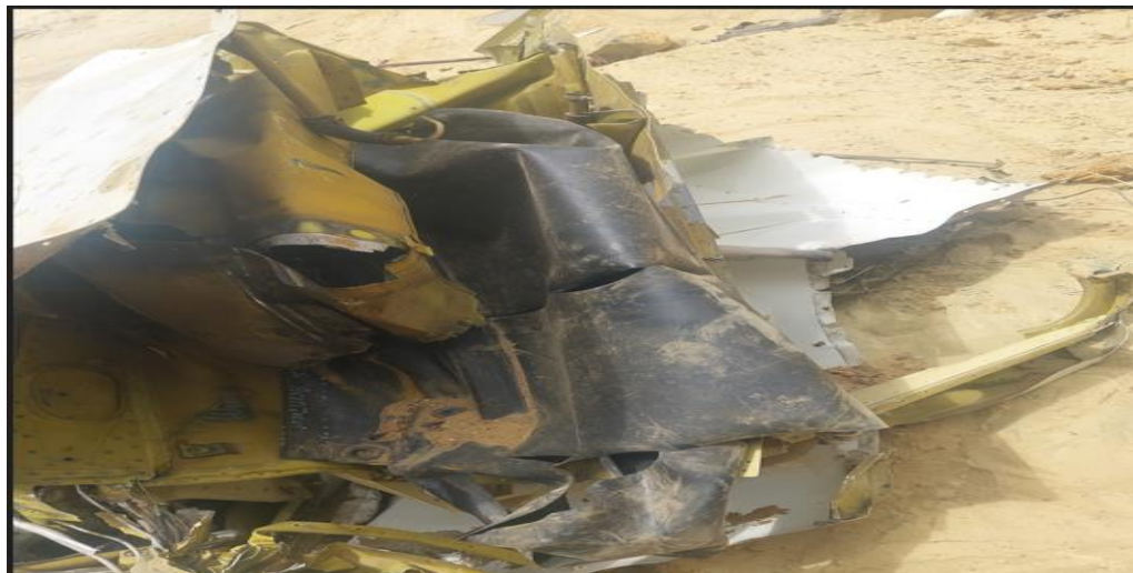
Figure 10: The ruptured fuel bladder tanks.
