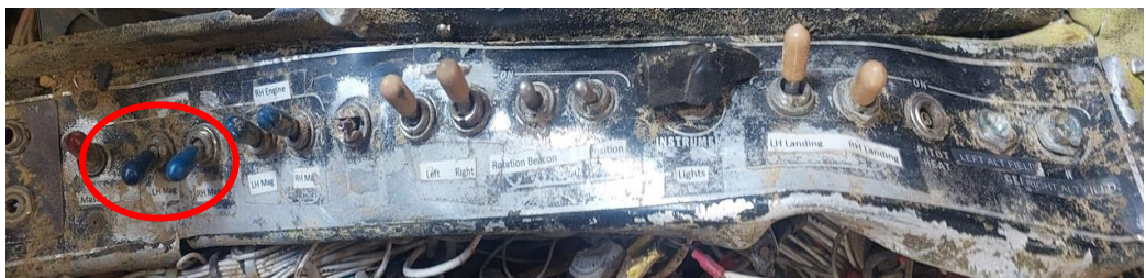
Figure 6: The cockpit instrument with the left-side magneto switch in the 'off' position.
