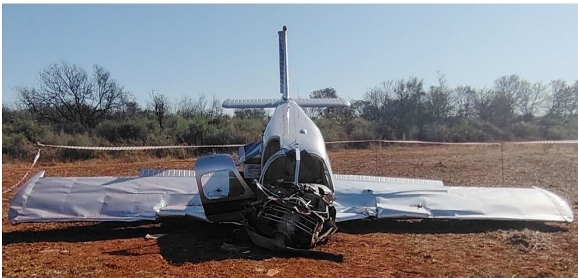
Figure 4: The damaged propeller and wings.
