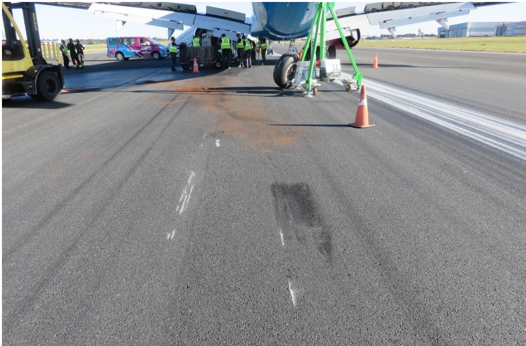
Figure 5: First markings on the runway surface caused by the brake assembly and the inner wheel rim when they contacted the runway.
