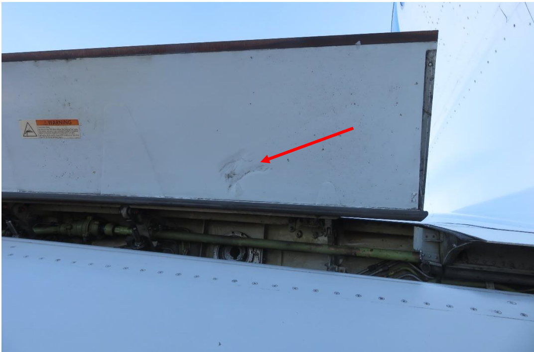
Figure 7: Damage on the inboard ground spoiler caused by the tyre debris.
