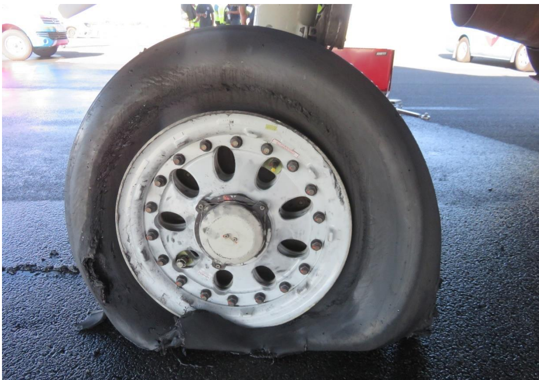
Figure 8: The left inner mainwheel tyre that burst during the landing roll.
