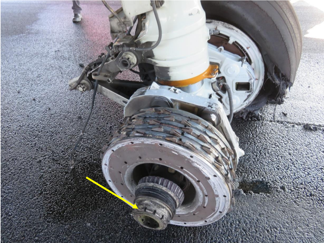
Figure 9: The left mainwheel brake assembly with the wheel nut still secured to the axle.
