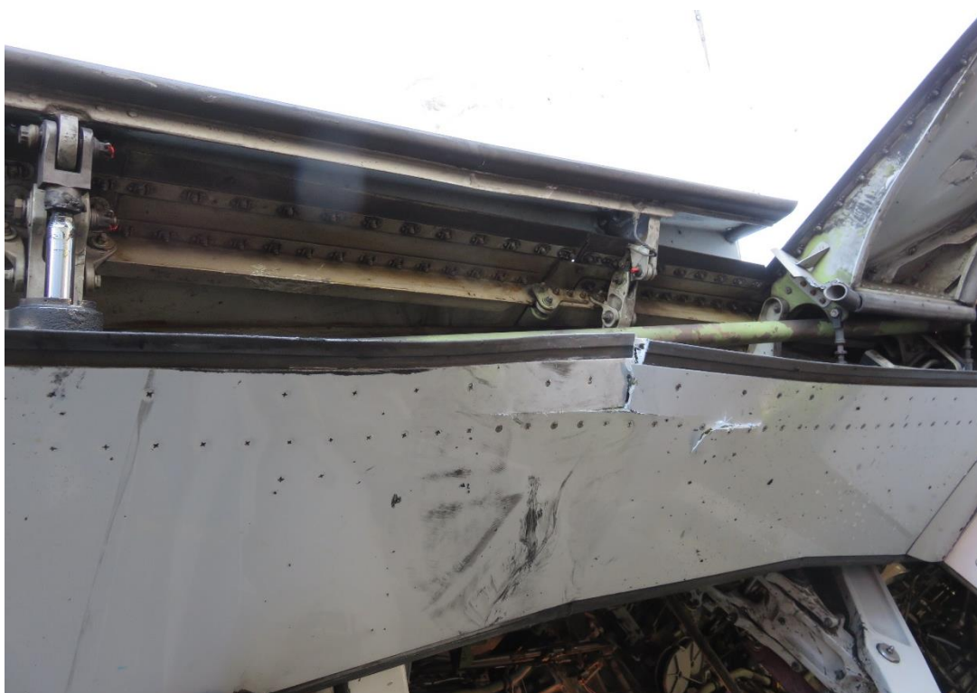
Figure 6: The ground spoiler protection fairing that was damaged by the tyre debris.
