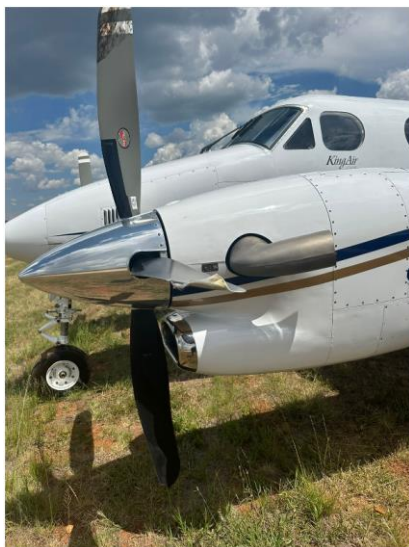
Figures 3 and 4: Damage to the No.1 engine propeller blades (left) and the left-side wheel assembly hubs (right).
