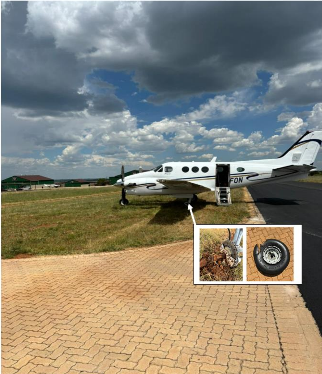
Figure 5: Damaged tyre struck by the propeller blades. (Source: Pilot)
