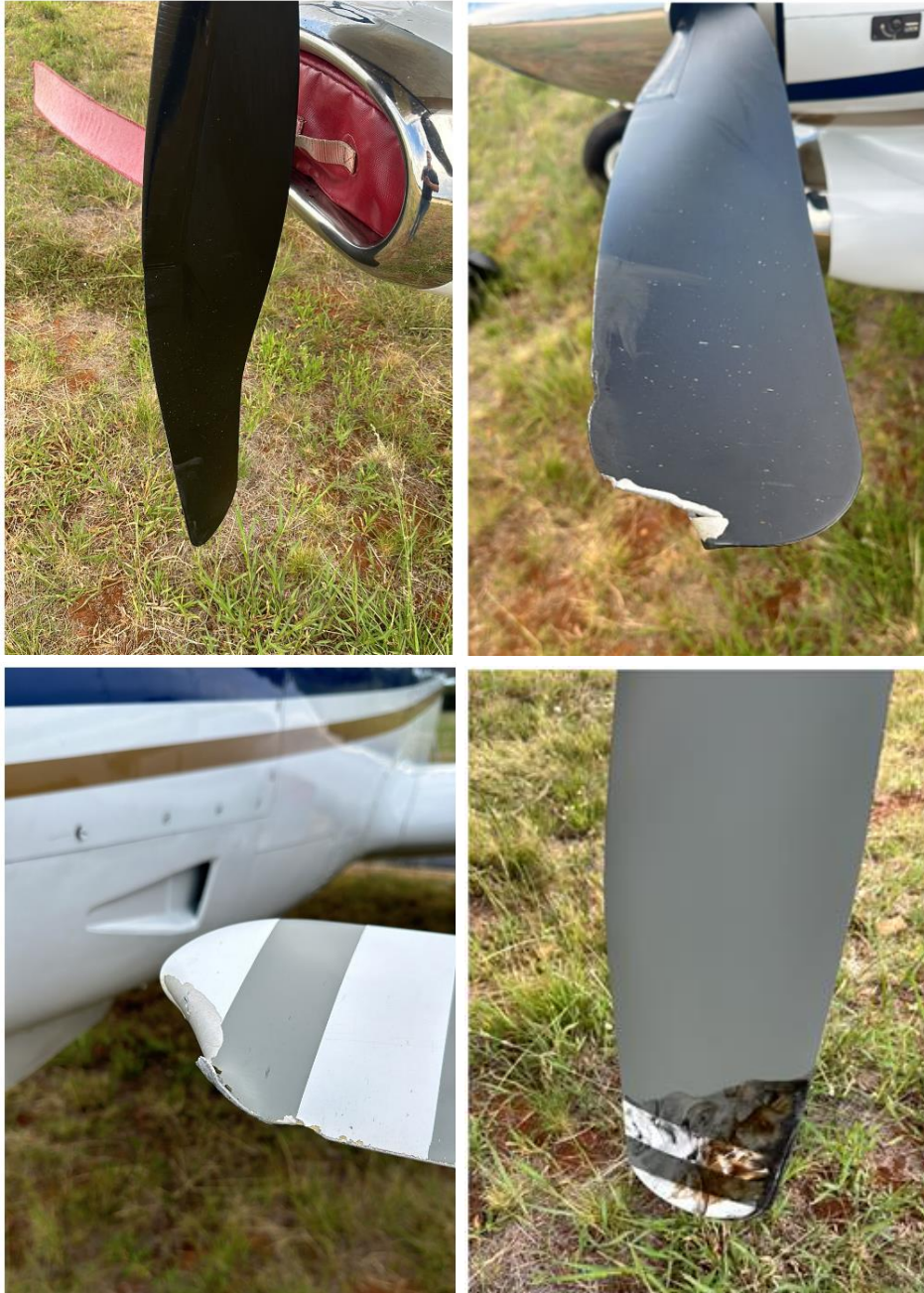
Figures 6, 7, 8 and 9: Damage sustained to the four (4) propeller blades. (Source: Pilot)
