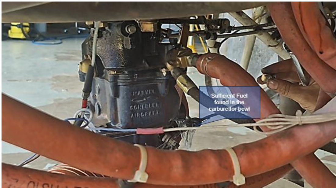
Figure 7: Snapshot of fuel found in the carburettor bowl.
