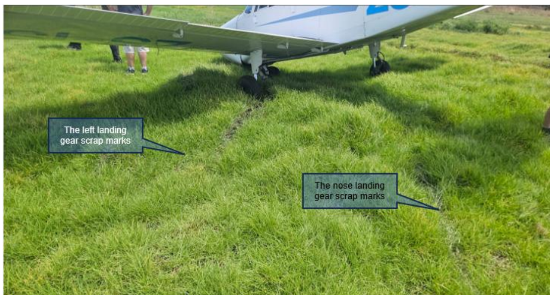
Figure 6: Shows the landing gear scrape marks over the embankment
