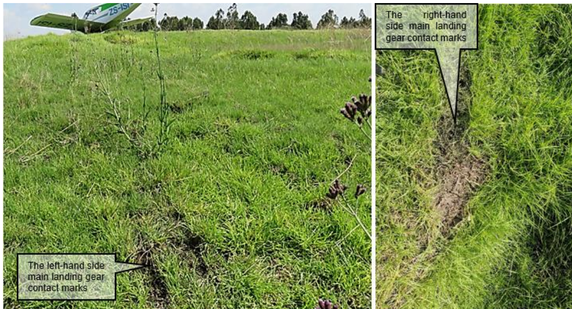
Figure 5: The initial impact marks of the left and right main landing gear.
