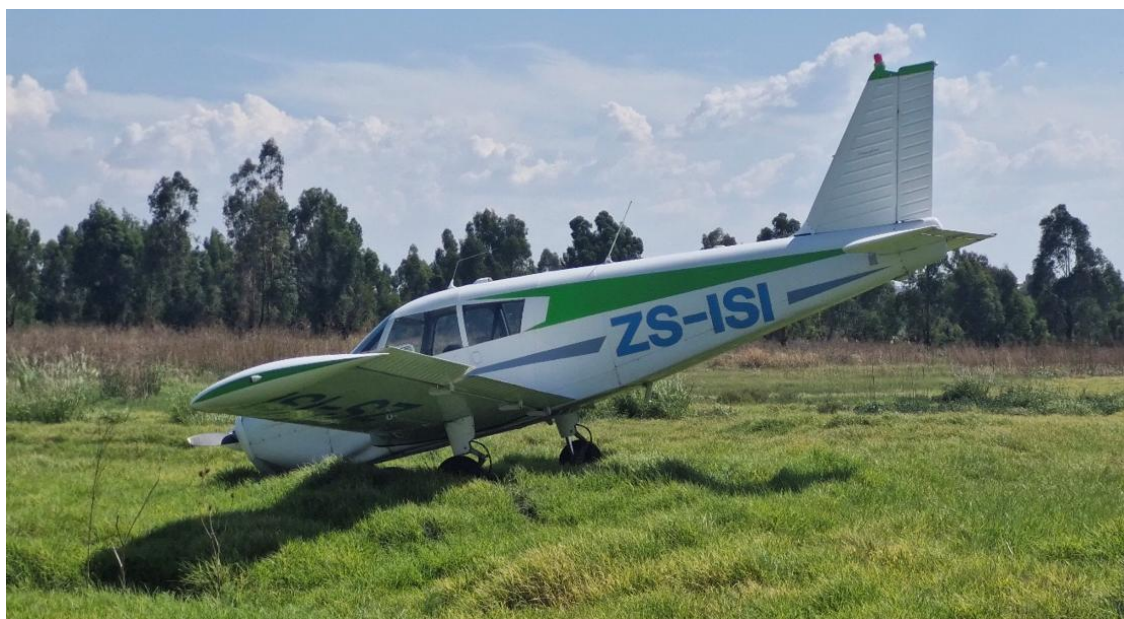
Figure 3: The aircraft as it came to a full stop with the damaged nose landing gear.
