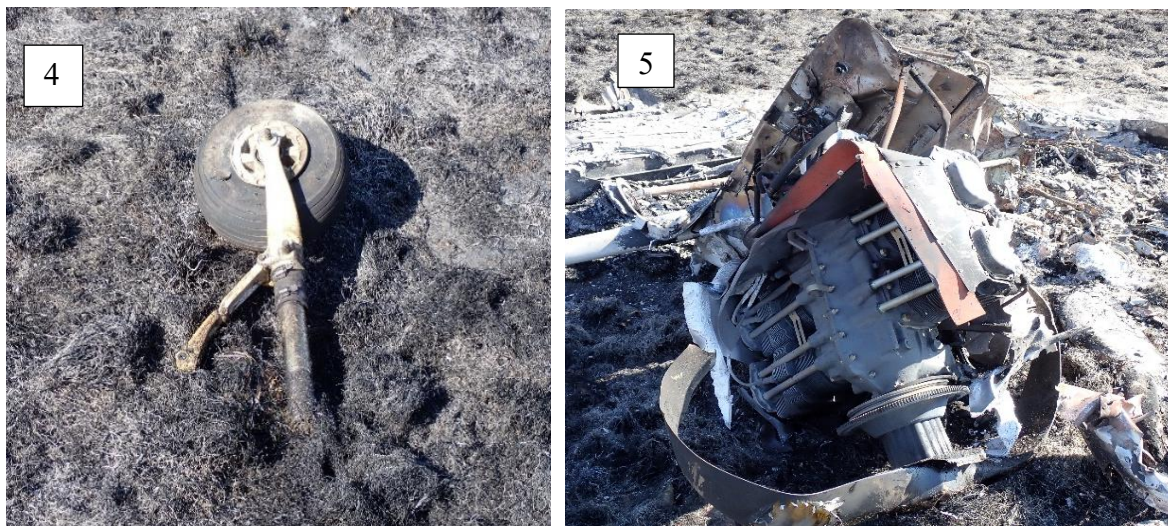
Figures 4 and 5: The nose landing gear and the engine casing were not scorched by the fire.
