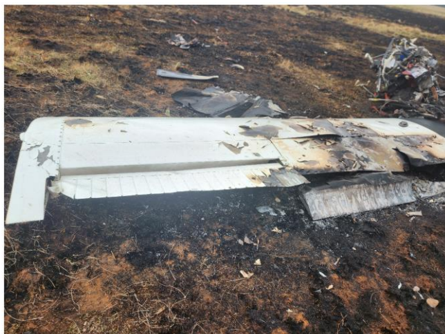
Figures 6 and 7: The damaged outboard (left) and inboard (right) of the left wing.
