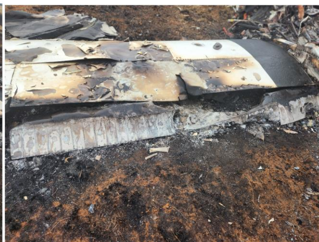
Figures 6 and 7: The damaged outboard (left) and inboard (right) of the left wing.
