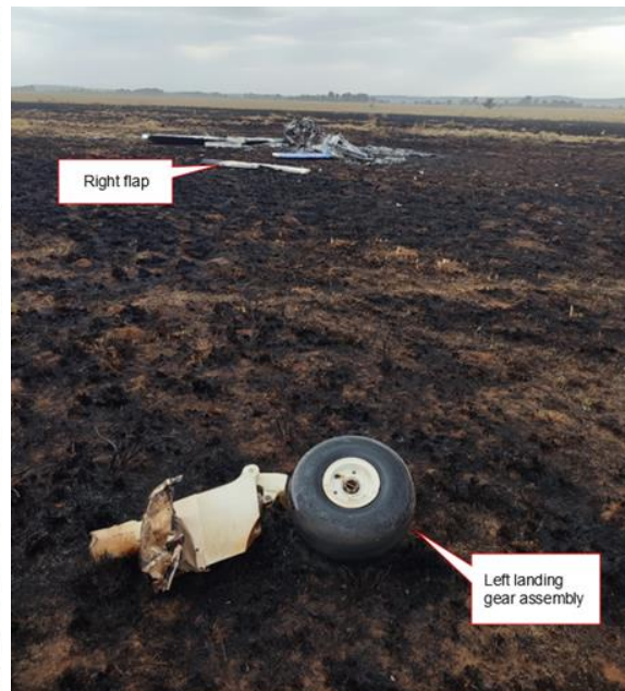
Figures 4 and 5: The right main landing gear assembly (left); and the left main landing gear assembly with rear view of the main wreckage in the background (right).
