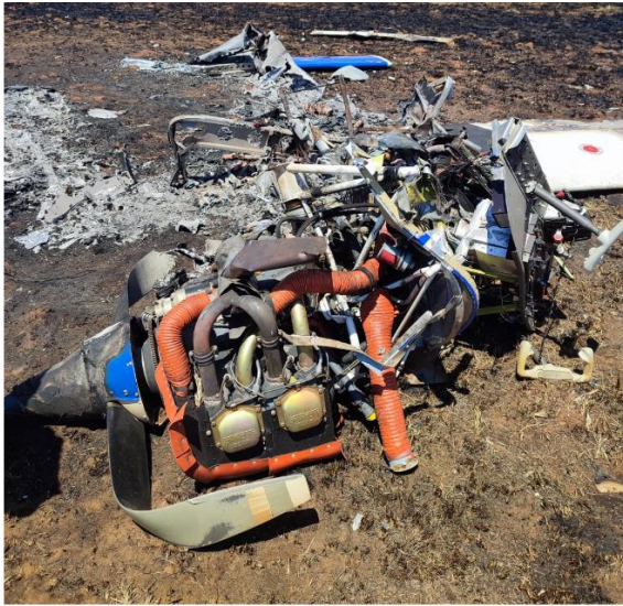
Figures 8 and 9: The damaged engine (left) and instrument panel (right).
